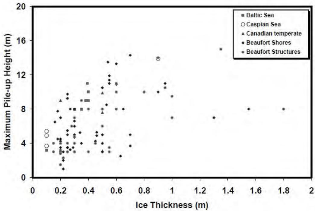
**Figure 19. Maximum Pile-Up Height vs. Ice Thickness from Full-Scale and Model Test Data (Timco and Barker, 2002)**
