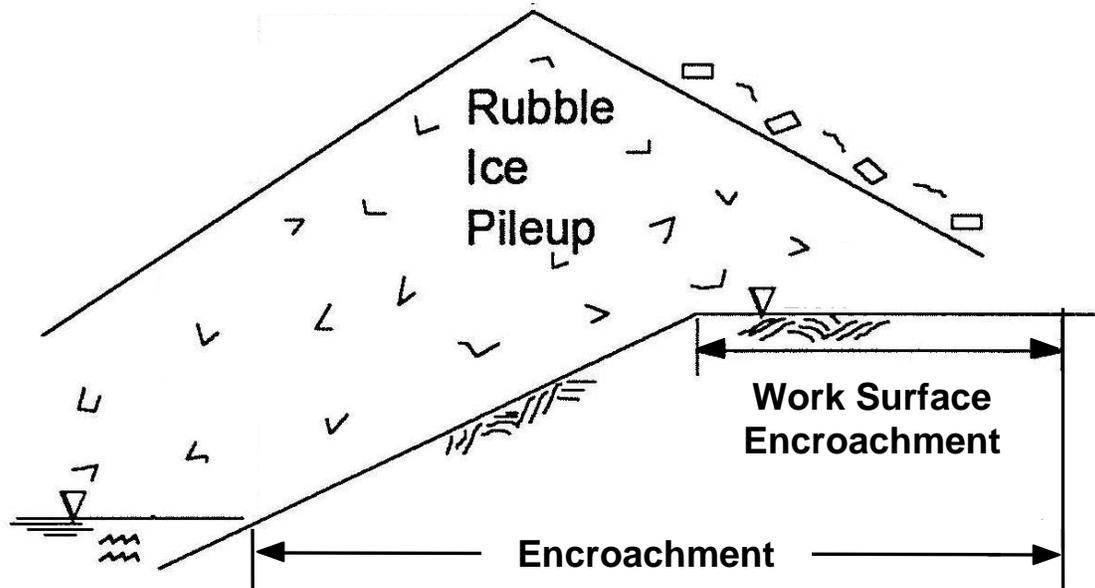
**Figure 14. Schematic Representation of Encroachment Resulting from Ice Pile-Up**
