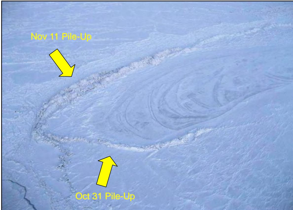
**Plate 27. 4-m Pile-Up that Formed on Southwest Side of Narwhal Is. on Oct. 31, 2011, and 7.6-m Pile-Up that Formed on Northwest Side on Nov. 13, 2011 (20-cm thick ice blocks encroached 4 m during 20- to 25-kt southwesterly storm in October; 30-cm thick ice blocks encroached 20 m during 15- to 25-kt westerly storm in November.)**
