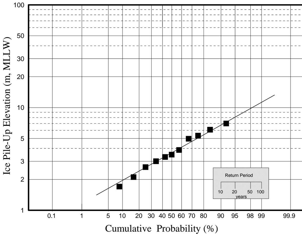
**Figure 17. Predicted Ice Pile-Up Elevations on Sheltered Natural Shorelines**
