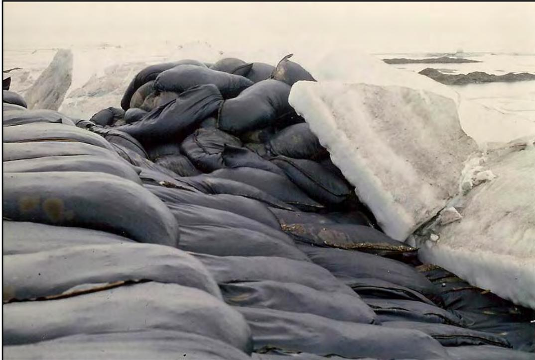
**Plate 30. Gravel Bags at Waterline of Tern Island Damaged by Ice Encroachment on June 30, 1982**
