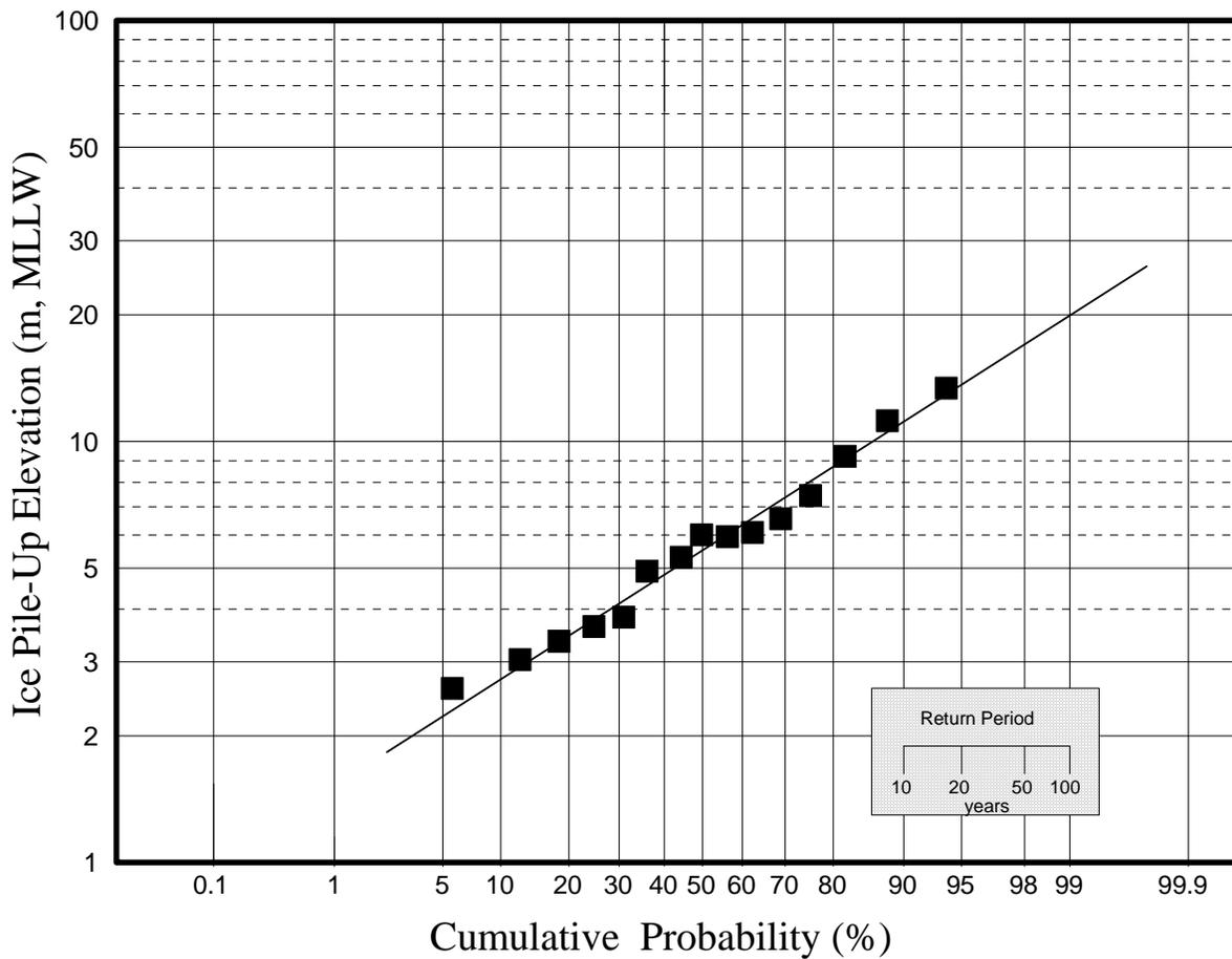
**Figure 16. Predicted Ice Pile-Up Elevations on Exposed Man-Made Facilities**
