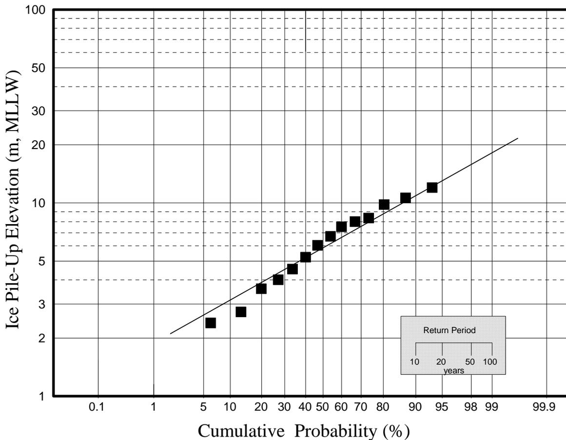
**Figure 18. Predicted Ice Pile-Up Elevations on Exposed Natural Shorelines**
