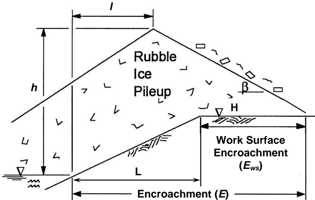
Figure 20. Geometric Parameters Used in Predicting Encroachment
