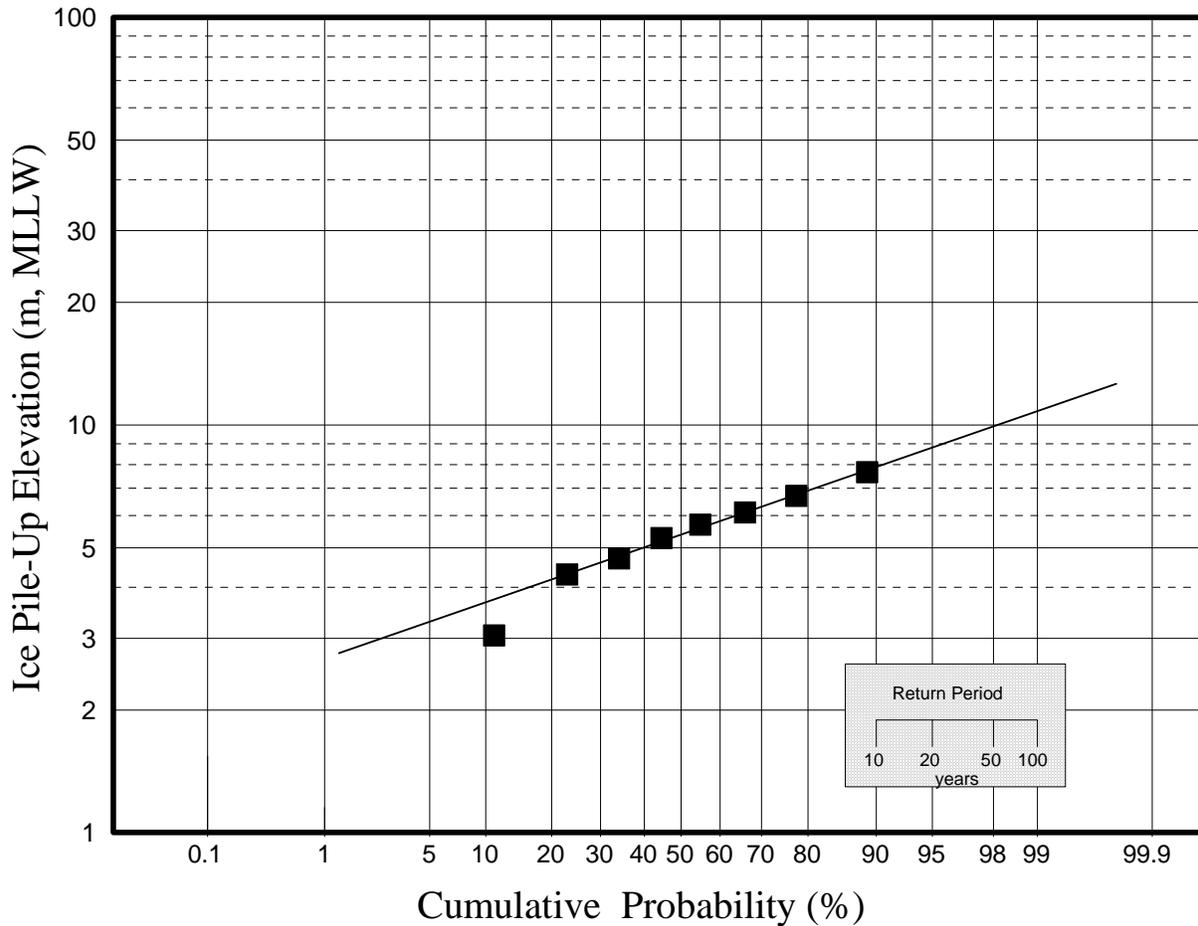
**Figure 15. Predicted Ice Pile-Up Elevations on Sheltered Man-Made Facilities**
