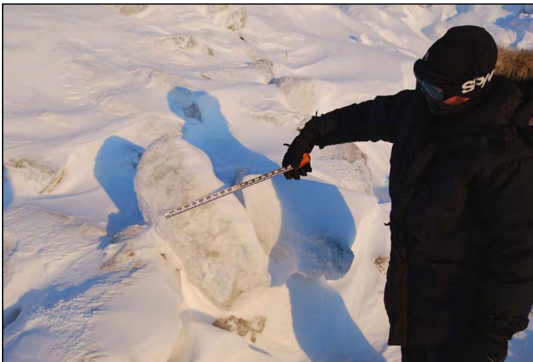
Plate 22. 30-cm Thick Ice Blocks Comprising 7.6-m Pile-Up on Narwhal Island (February 4, 2012)
