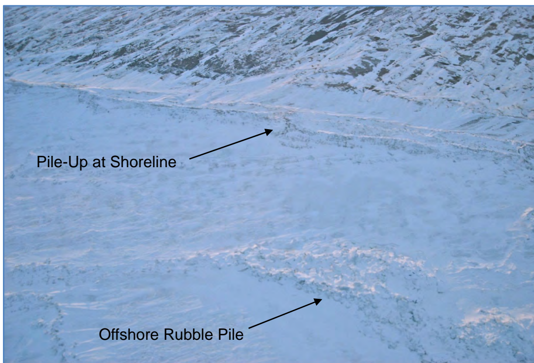
Plate 44. 12-m High Ice Pile-Up with Offshore Rubble Pile at Icy Cape (February 6, 2012)
