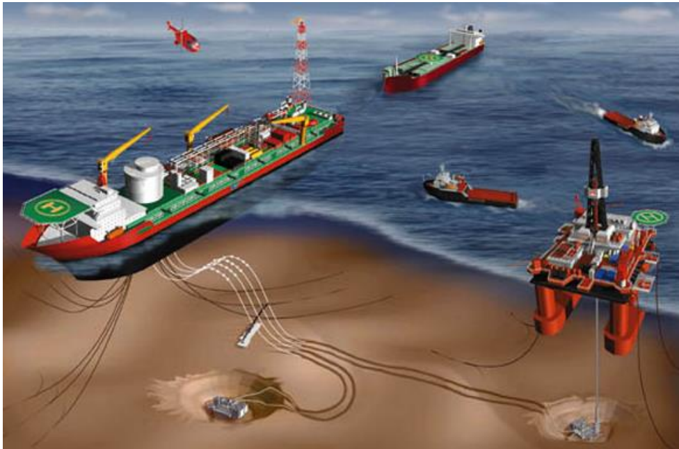
Figure 2.19: Mud Cellars in the Terra Nova Field
