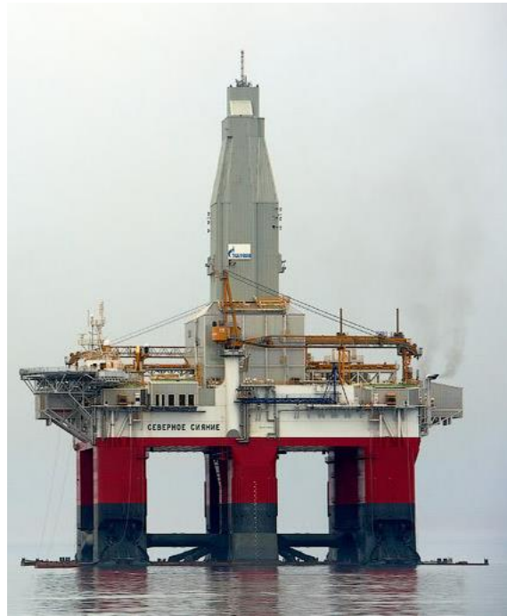
Figure 2.10: Northern Lights (Semi-submersible Vessel)
