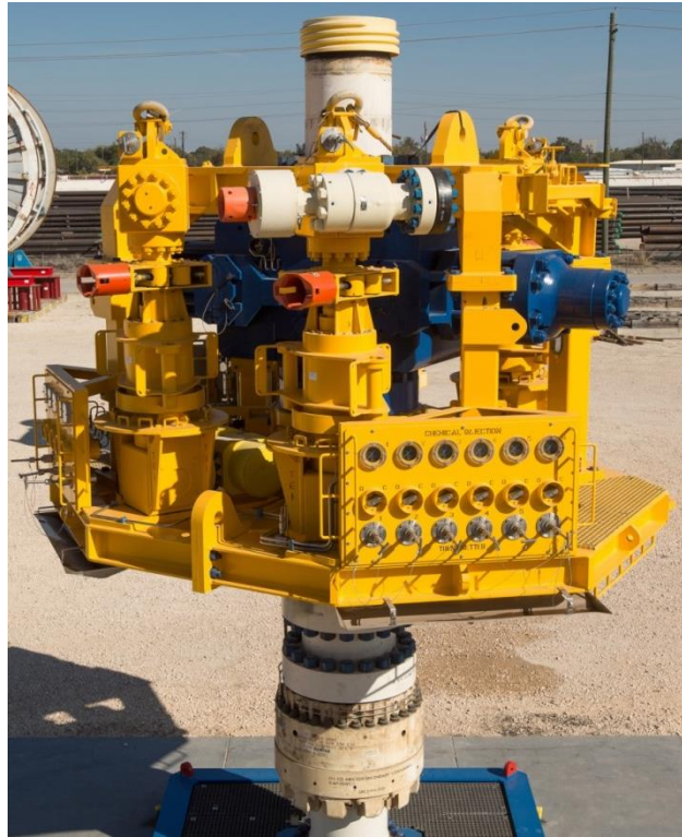
Figure 2.1: 15,000-psi Subsea Capping Stack [2]
