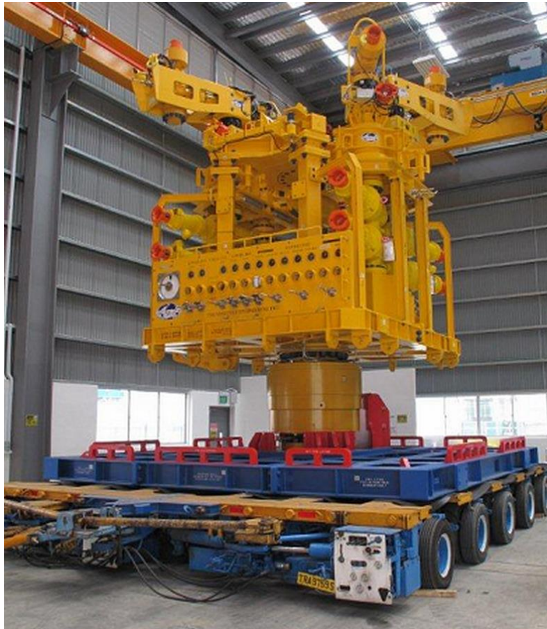
Figure 8.3: OSRL Subsea Capping Stack Stored on Towable Trolley [17]
