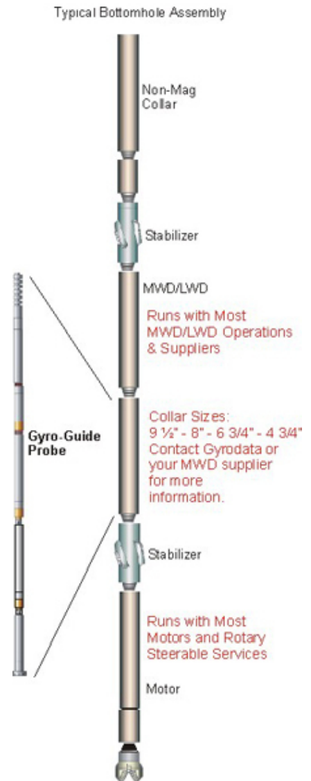
Figure 1: Typical BHA Configuration with MWD & GMWD (from: Gyrodata Inc. reproduced with permission)
