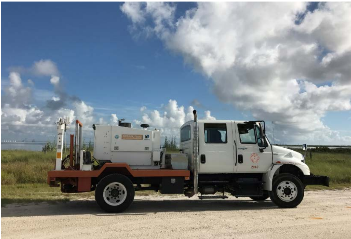
Figure 3.31 Shaker truck “Thumper” used in in-situ dynamic tests (Site 1 and Site 2)
