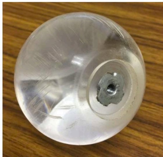
Figure 4.7 Sphere recessed cavity and connection to load cell
