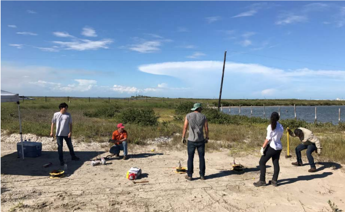
Figure 3.32 Generating waves using sledgehammer at Site 3
