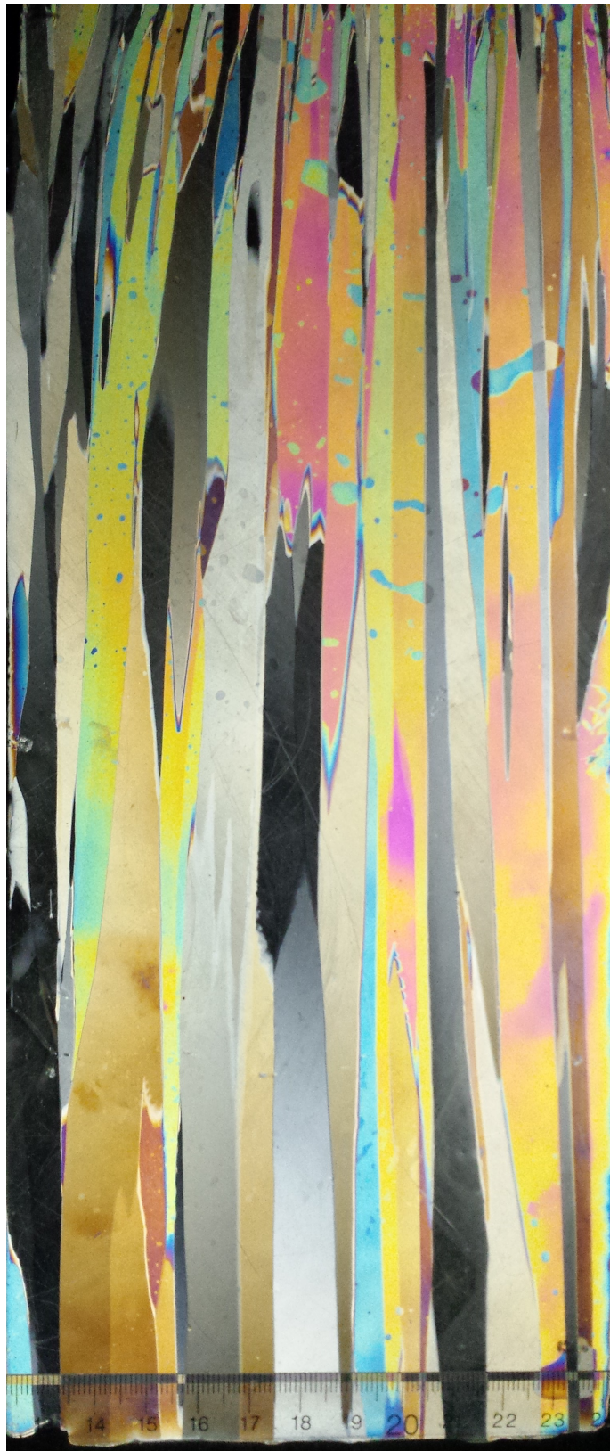
Figure 3: Photograph of a vertically-oriented thin-section (~1mm) of columnar-grained, freshwater ice as viewed between crossed-polarized filters.
