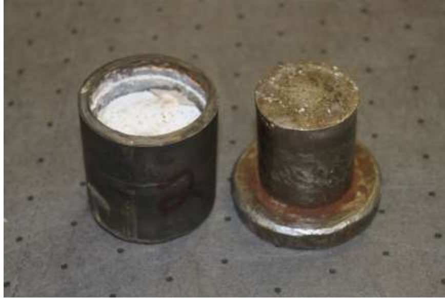
Figure 35: Shear Bond Test Apparatus
