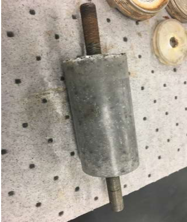
Figure 39: Tensile Modulus Test Specimen
