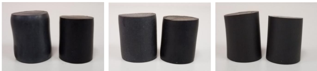
NBR @120°F: Vapor (left), Brine (right)
