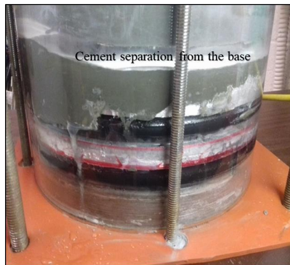
Figure 4.25: Cement separation during the 20-psi pressure test.
