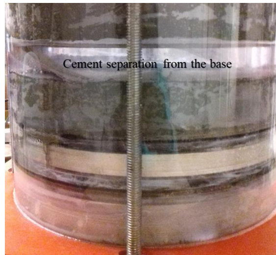
Figure 4.17: Cement separation during the 40-psi pressure test.
