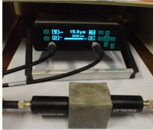
Figure 2.46: Ultrasonic cement test being carried out.
