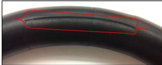
Figure 4.8: Elastomer after creating a seam as an intentional physical defect
