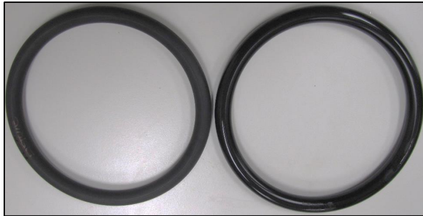
Figure 4.5: EPDM elastomers before (left) and after (right) degradation with surfactant.
