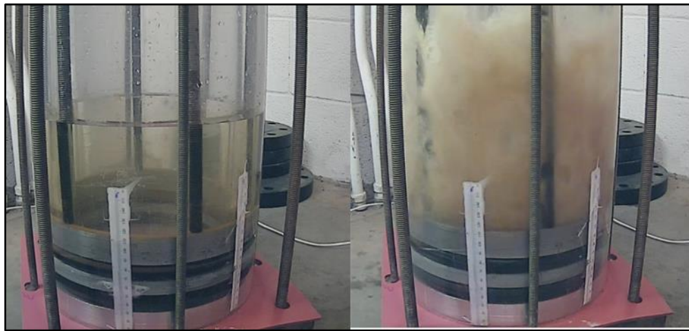
Figure 4.16: NBR pressure cycling test at 180 in-lbf and 120 in-lbf (successful tests).
