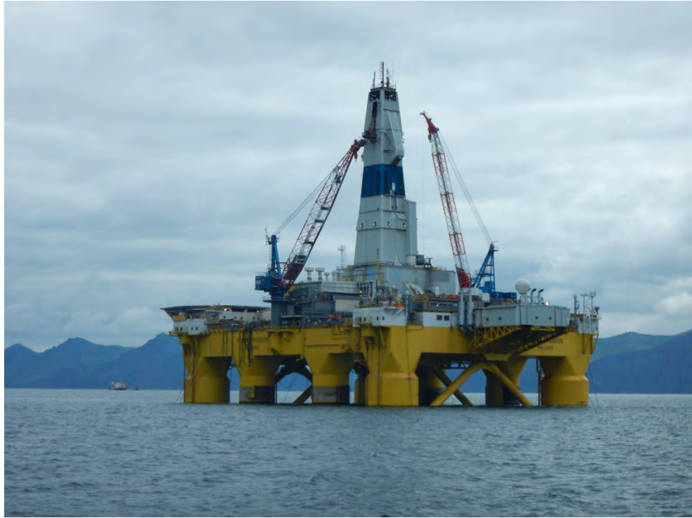
Figure 4-5. Example of a semi-submersible drilling vessel, Polar Pioneer (US BSEE, 2018).
