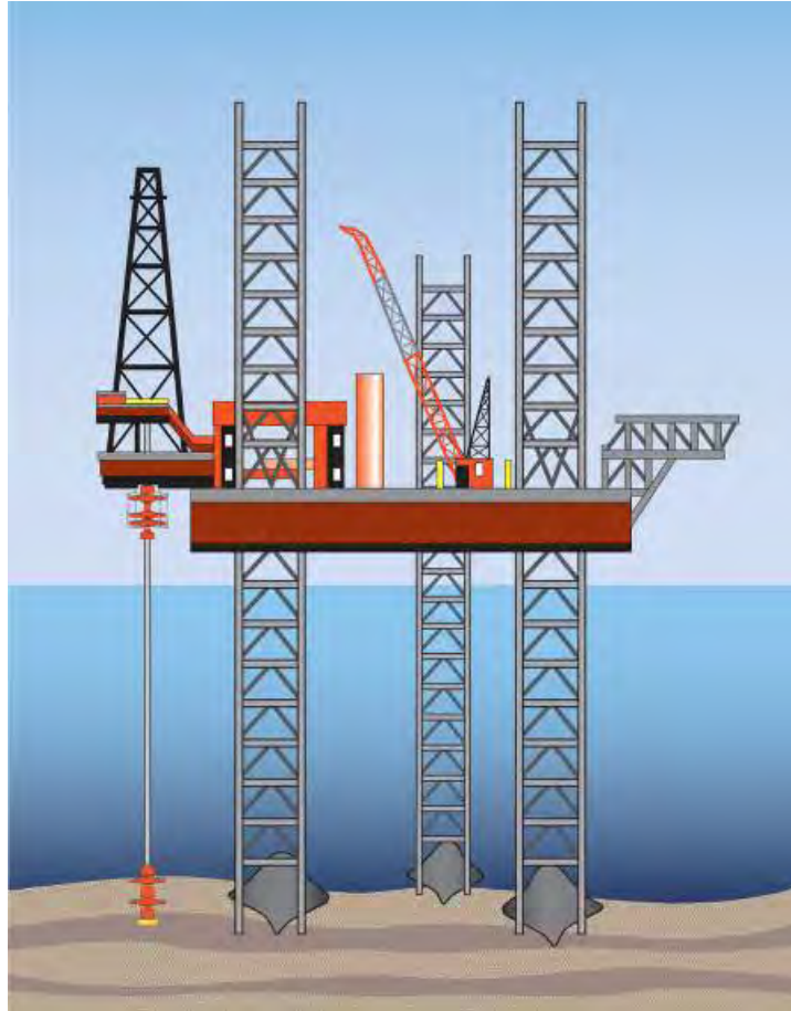
Figure 4-4. Example of a jackup drilling rig with SID on seafloor (Faust, 2012).
