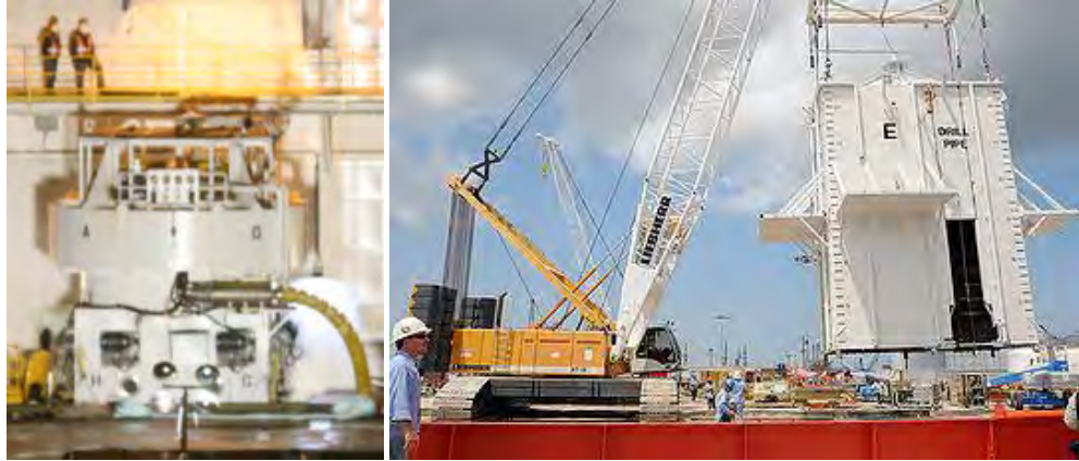
Figure 4-1. Examples of containment domes for Shell Arctic and the Macondo response.
