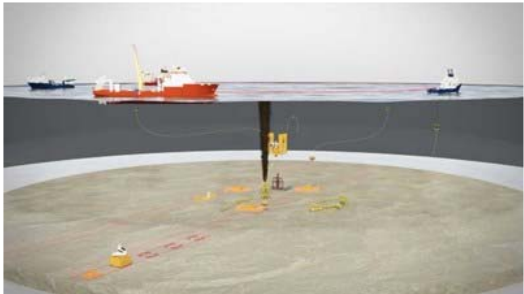
Figure 3-6. OSRL offset SCCE installation system (OSRL, 2018).
