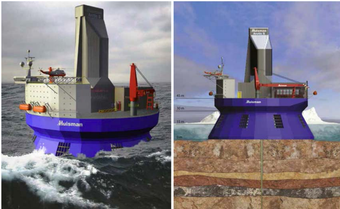
Figure 1-4. Huisman Arctic S drilling vessel concept design (Huisman, 2018).
