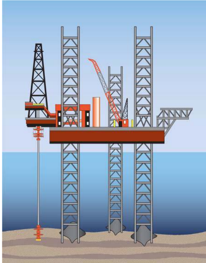
Figure 3-8. Jackup drilling vessel with SID installed near the seafloor (Faust, 2012).
