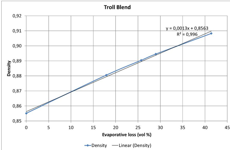
The relation between density and evaporation for the Alaska North Slope crude oil that was used in the tests was based on analysis of samples artificially weathered in a wind tunnel. The relationship between evaporative loss and density for ANS is shown below.
