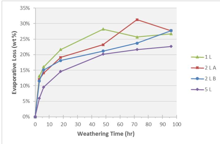
Figure 3-2: Evaporative loss over time for ANS crude oil
