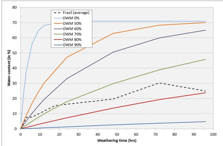
Figure 3-9: Water content of ANS in 96-hr flume experiments and model predictions with varying ice coverage
