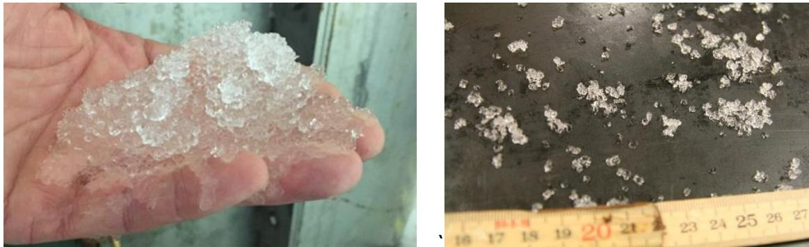
Figure 2-3: Frazil ice produced at SINTEF
