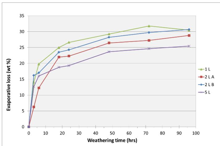
Figure 3-1: Evaporative loss over time for Troll Blend crude oil
