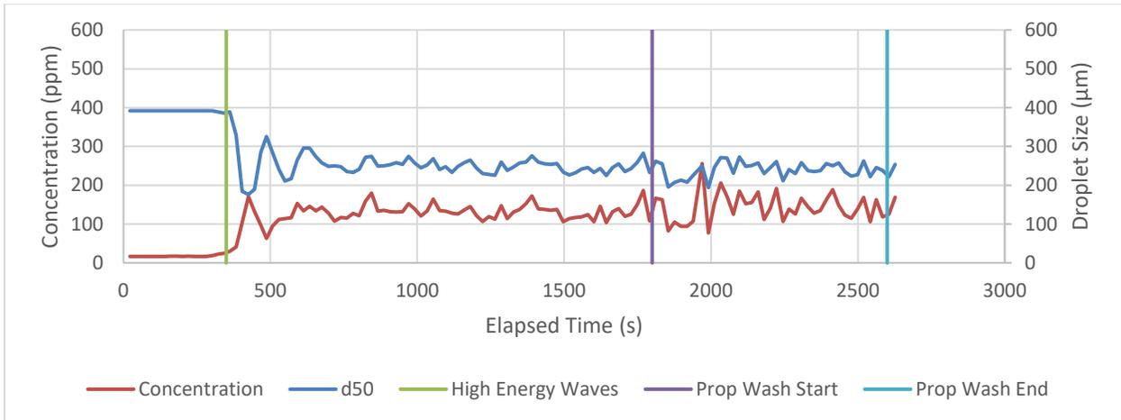
Figure 3-22: 1 L Weathered Troll Blend in 10 cm of Frazil Ice
