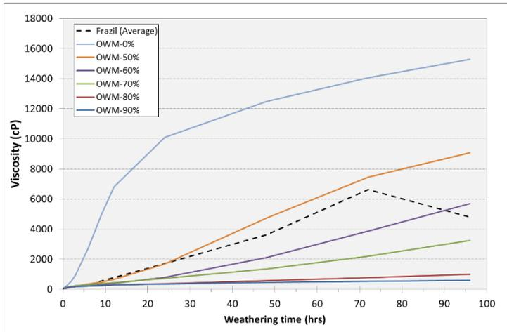
Figure 3-11: Viscosity of ANS from 96-hr flume experiments and model predictions with varying ice coverage
