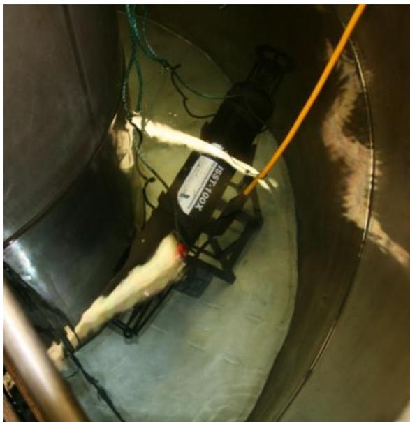
Figure 2-2: LISST 100X Type C, mounted in flume
