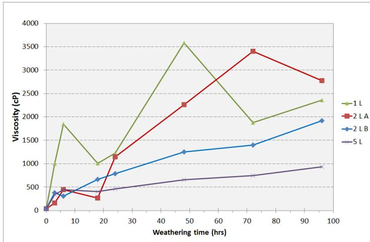
Figure 3-5: Viscosity over time for Troll Blend crude oil
