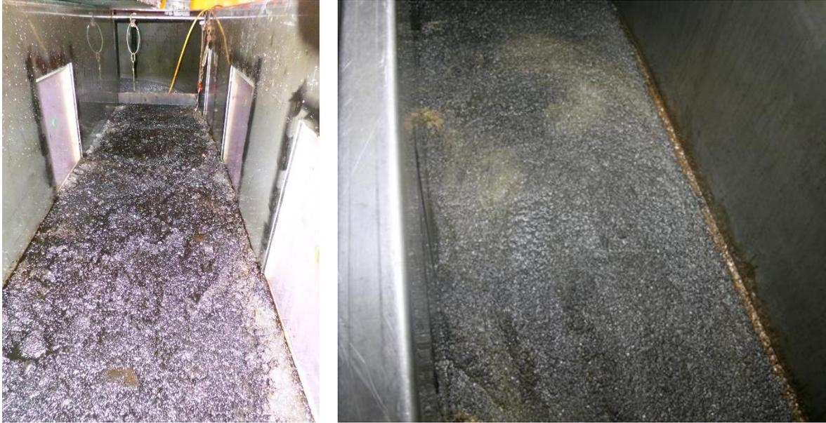
Figure 2-5: ANS crude oil and ice in the SL Ross flume tank (left) and Troll Blend crude oil in the SINTEF flume tank (right).
