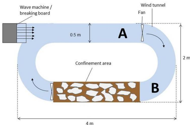
Figure 2-1: Sketch of SINTEF and SL Ross meso-scale recirculating flumes.
