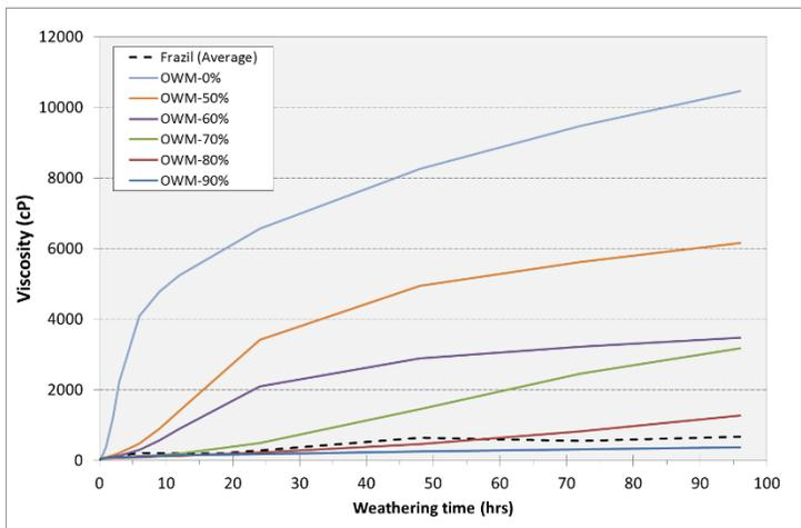
Figure 3-12: Viscosity of Troll Blend from 96-hr flume experiments and model predictions with varying ice coverage
