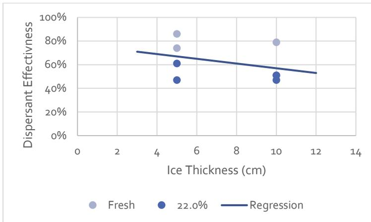
Figure 3-15: Dispersant effectiveness with ice thickness for Troll Blend crude oil
