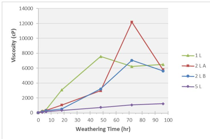
Figure 3-6: Viscosity over time for ANS crude oil
