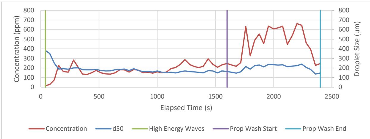
Figure 3-23: 2 L Weathered Troll Blend in 10 cm of Frazil Ice
