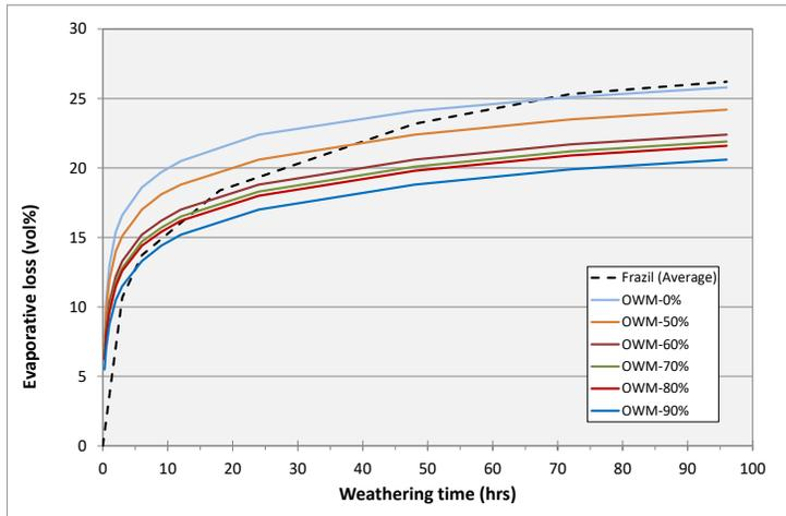
Figure 3-7: Evaporative loss of ANS in 96-hr flume tests and model predictions with varying ice coverage
