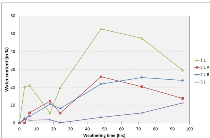
Figure 3-3: Water content over time for Troll Blend crude oil
