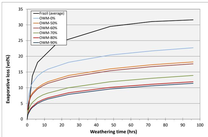
Figure 3-8: Evaporative loss of Troll Blend in 96-hr flume experiments and model predictions with varying ice coverage
