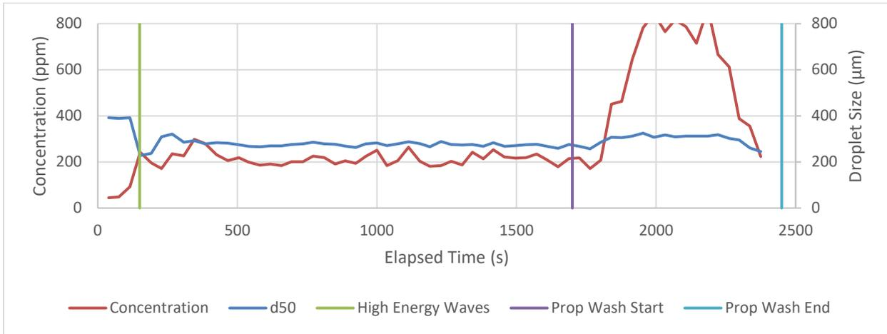
Figure 3-19: 1 L Weathered Troll Blend in 5 cm of Frazil Ice
