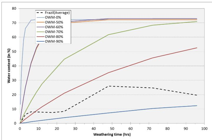
Figure 3-10: Water content of Troll Blend in 96-hr flume experiments and model predictions with varying ice coverage
