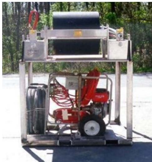
Fig. 85-Action Petroleum Spill Recovery Inc. Model 24 Drum Skimmer. Photographed with power unit on storage cart [66].
