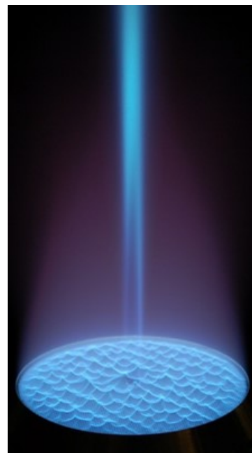
Fig. 14- Laboratory spray burner operation with heptane spray.
