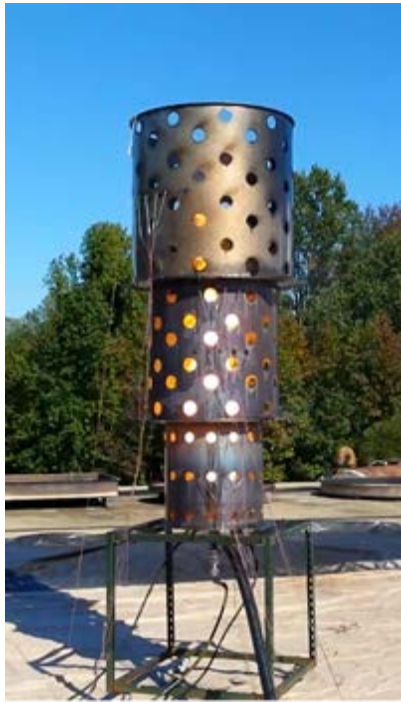
Fig. 43-Photograph of the engineering-scale burner during operation, burning Oriente crude oil.
