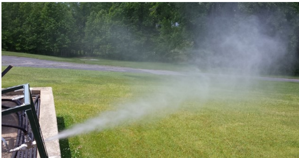
Fig. 36-Photograph of the LFBA atomizer test at an ALR = 0.91, performed at CBD. Airflow was 3.2 \times 10^{-2} kg/s and the water flow rate was 2.1 L/min, or 3.5 \times 10^{-2} kg/s.
