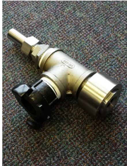
Fig. 10-Photograph of the assembled atomizer for the engineering-scale burner.
