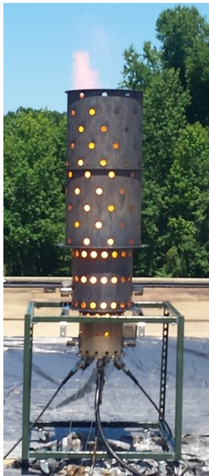
Fig. 41-Reconfigured burner burning an assumed-50% emulsified crude oil, with an air flow of 1.60 \times 10^{-2} kg/s and a liquid flow rate of 0.75 L/min, for an ALR of 1.32.
