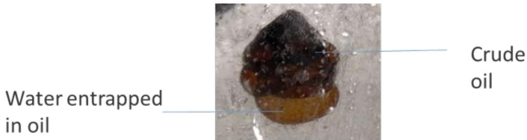
Figure 25. Water-in-oil emulsion was found in flotation operation.
