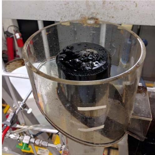
Figure 23. Typical oil overflows from the top of flotation column.
