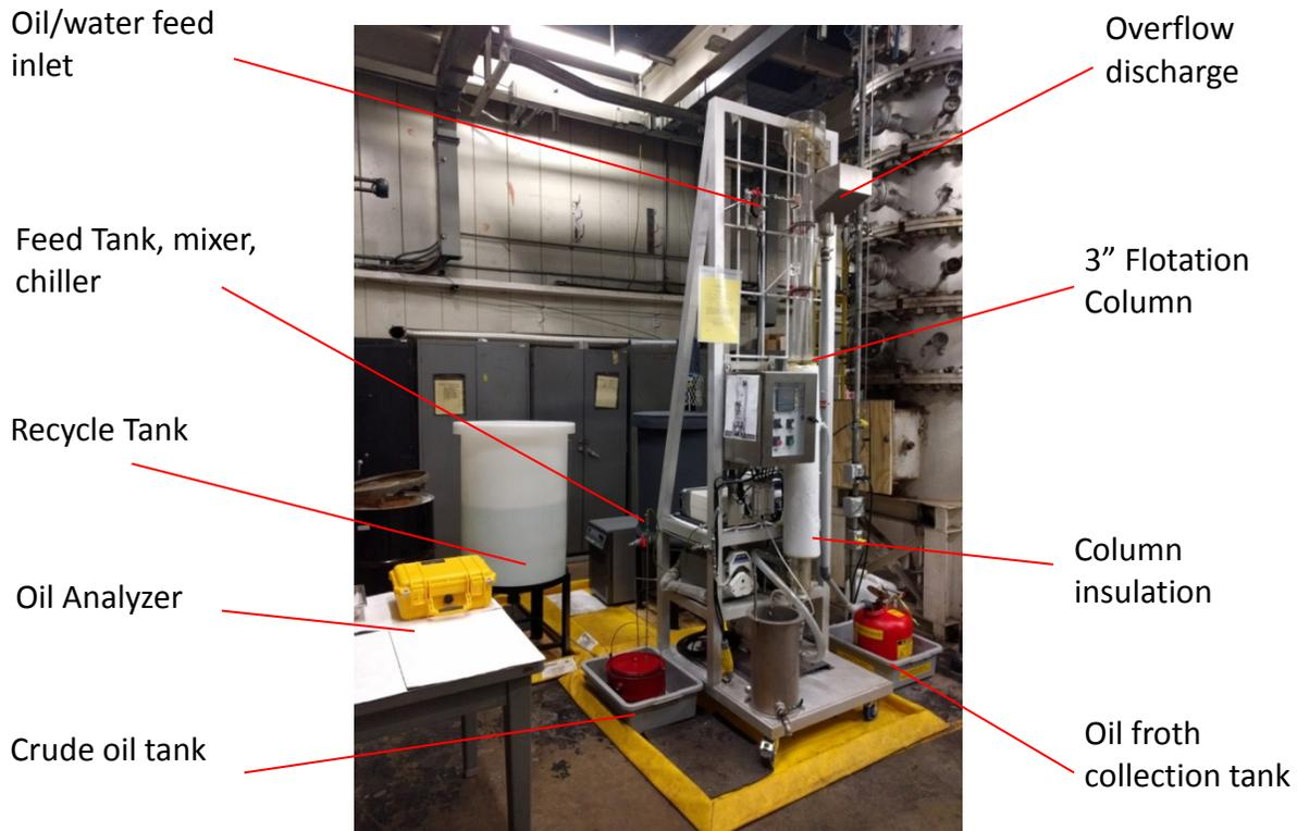
Figure 21. A 3" flotation column system for oil separation study.
