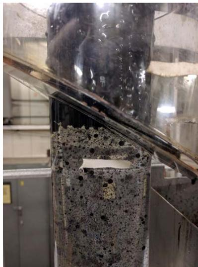
Figure 27. ANS crude in the presence of 10 ppm of Romax 6000 in flotation column at 5 °C.
