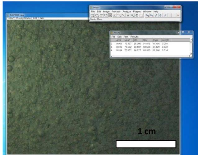
Figure 22. A digital image of gas bubbles analyzed using ImageJ 1.20.
