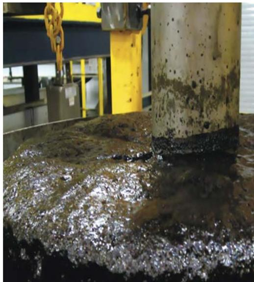
Figure 2. Oil separation using a Jameson flotation column; courtesy of Jameson Cell. <sup>[8]</sup>
