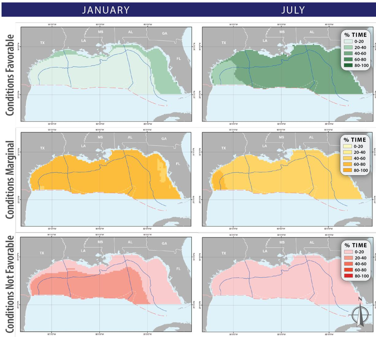
Figure 6-1. Selection of results maps for Mechanical Recovery – Two Vessels with Boom for January and July, representing the focus months in which conditions are most and least likely to be viable for this system across the study area
