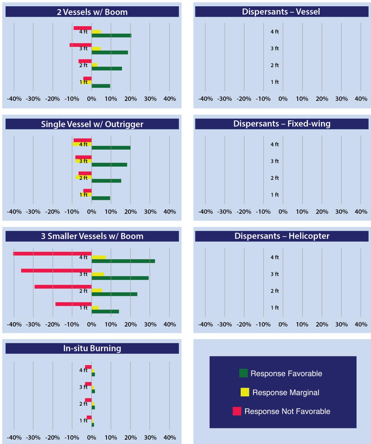
Figure 6-10. Percentage change in results from increasing tolerance to wave height by 1, 2, 3, and 4 feet as compared to the baseline results
