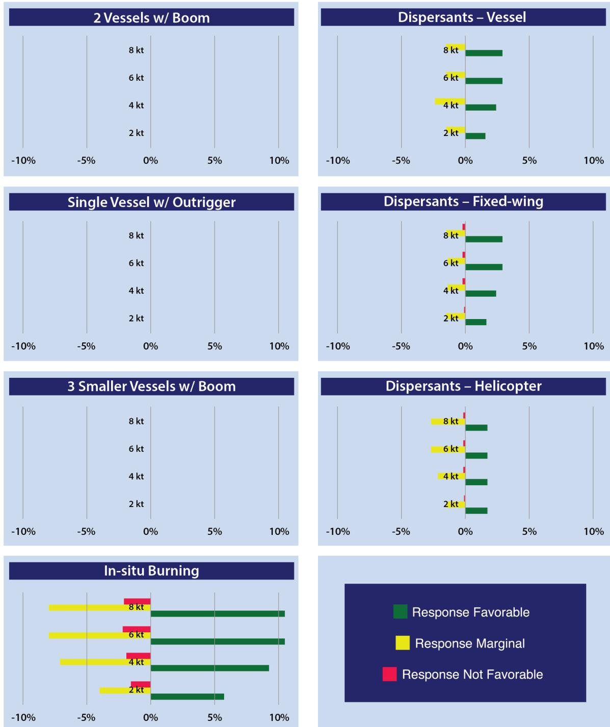
Figure 6-9. Percentage change in results from increasing tolerance to wind speed by 2, 4, 6, and 8 knots as compared to the baseline results
