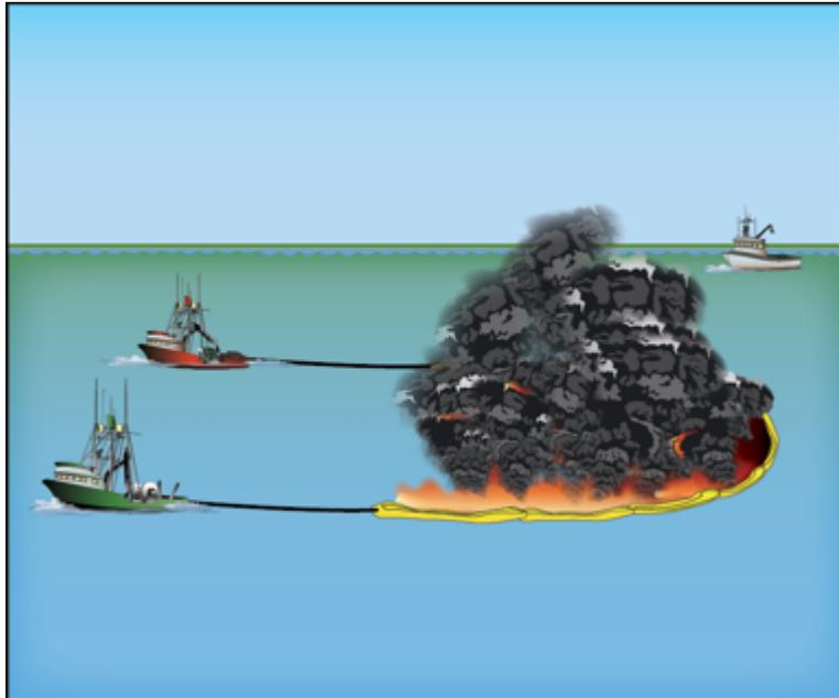
Figure 5-7. In-situ Burning – Vessels with Fire Boom
