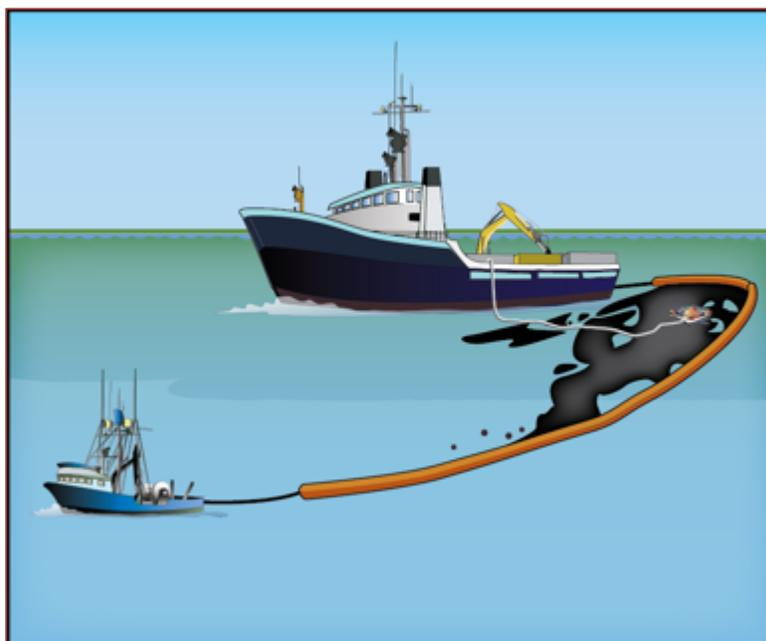
Figure 5-1. Mechanical Recovery – Two Vessels with Boom
