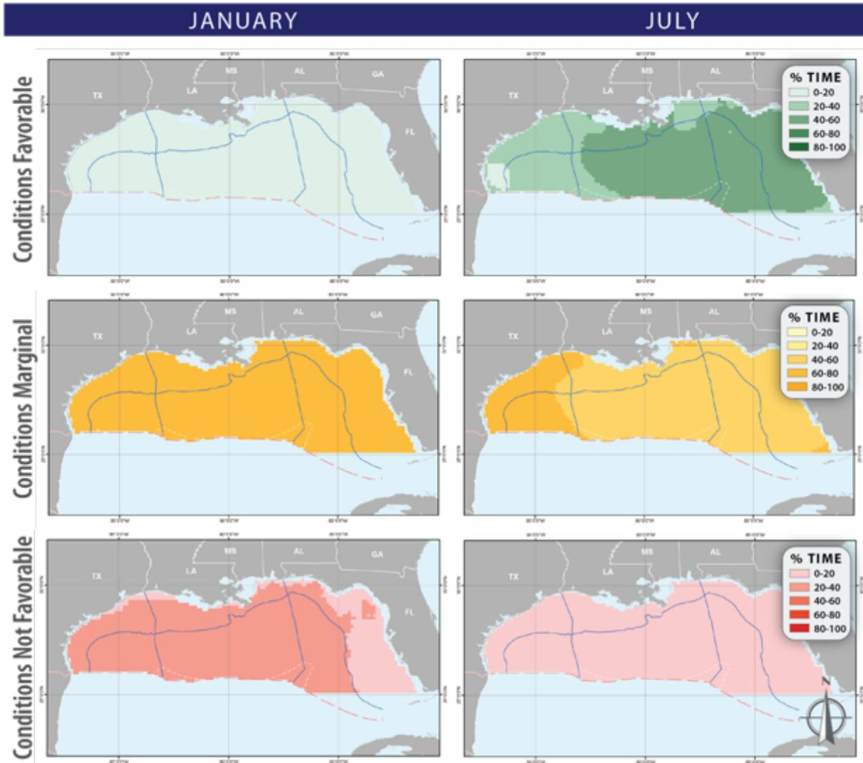
Figure 6-5. Results maps for In-situ Burning – Vessels with Fire Boom for January and July, representing the focus months in which conditions are most and least likely to be viable for this system across the study area
