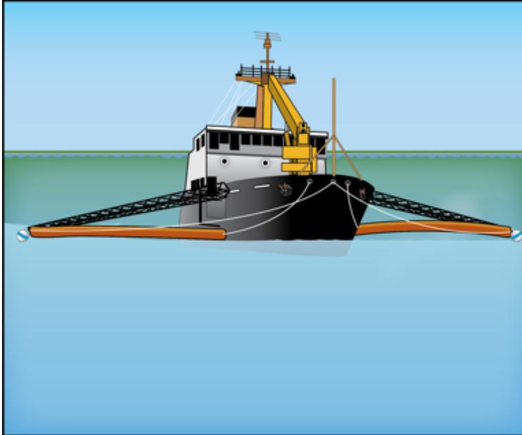
Figure 5-2. Mechanical Recovery – Single Vessel with Outrigger
