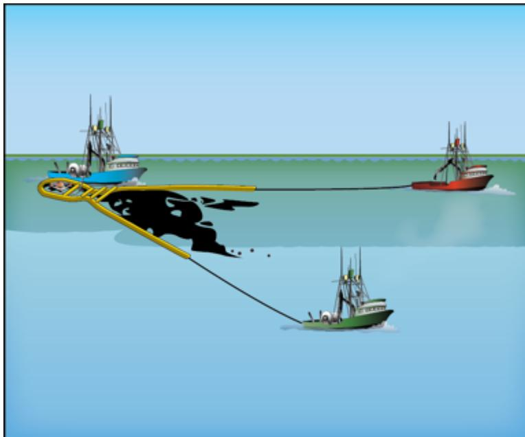
Figure 5-3. Mechanical Recovery – Three Smaller Vessels with Boom
