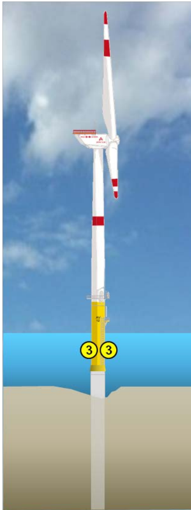
Figure 5-9 (Left) Positions of scour monitoring sonars on a mono pile foundation
