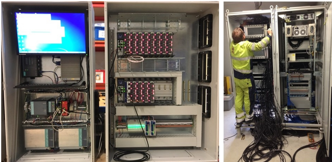
Figure 6-4 Large scale and modular SHM data acquisition system from NGI. Right, termination of strain gauges cables requires space and focus (Photo NGI archives)
