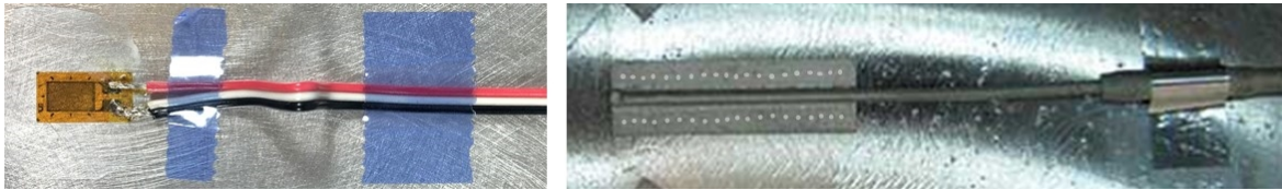
Figure 5-24 Glued Foil strain gauge (left) and micro spot welded strain gauge (right). Some models of spot welded strain gauges have the resistance wire protected inside a water and pressure resistant tube allowing them to be immersed in seawater
