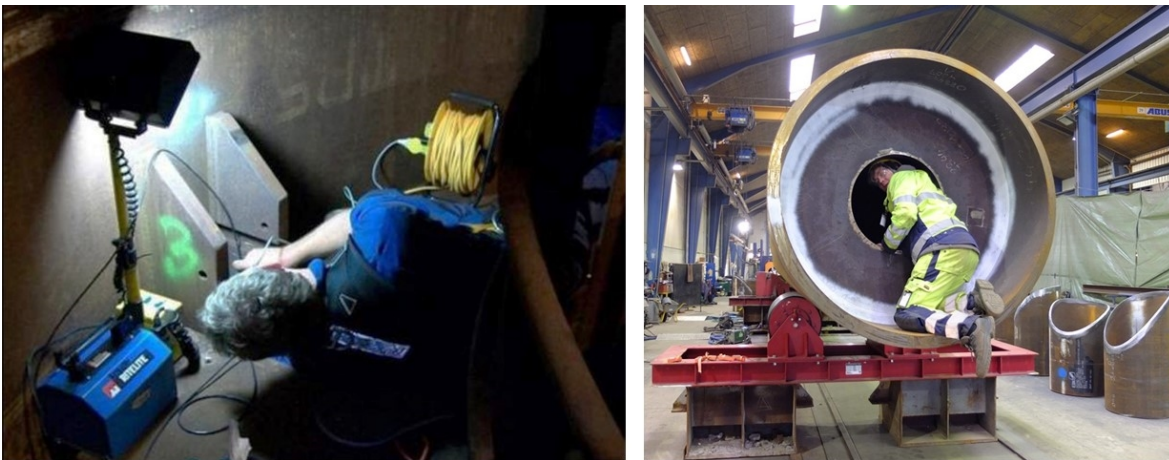
Figure 7-10 Left, darkness and confined space when installing extensometers inside the TP just above the sea water level (Photo: Strainstall) or right, when strain gauging a jacket leg (photo: NGI)
