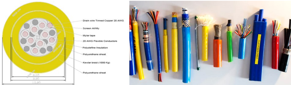
Figure 7-36 Typical cross section and examples Kevlar reinforced PUR cables for offshore and subsea use
