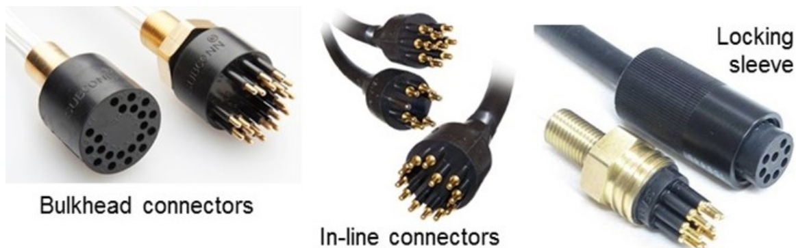
Figure 7-32 Neoprene bulkhead and inline connectors with over molded pin seals. Locking sleeve arrangement shown to the right. These types of connectors are not water blocked.
