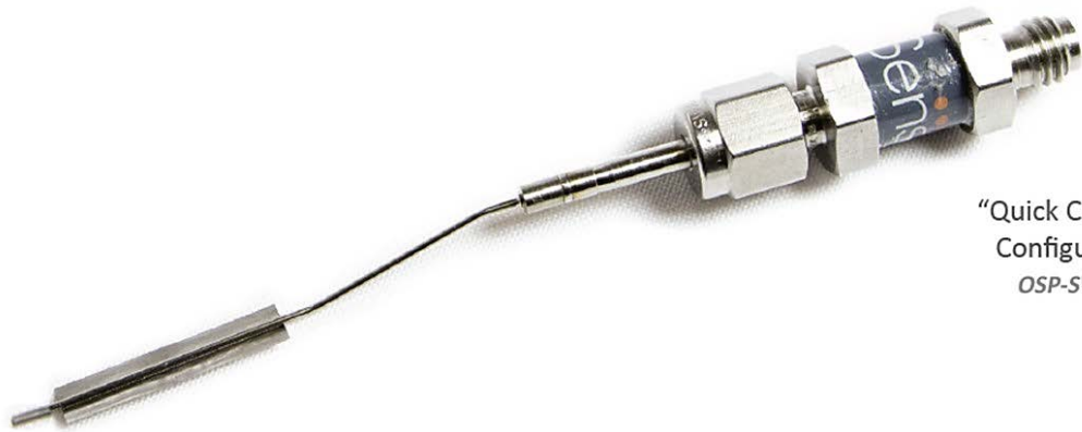
Figure 5-34 Weldable fiber optic strain gauge from Opsens based on Fabry Perot sensing principle and white light interferometry, fully submersible assembly with quick connector
