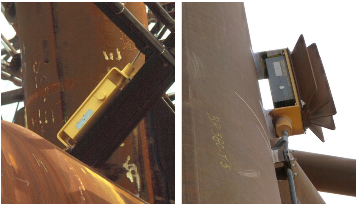
Figure 5-72 Permanent reference electrodes for external use from Polatrak, the (right) version is equipped with a 1m 2 current density monitor.
