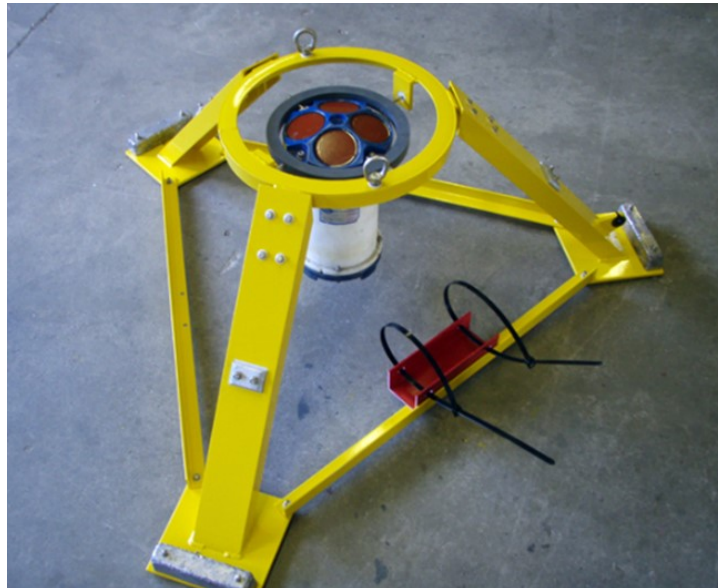
Figure 7-24 Coated bottom mount for ADCP sensor with zink anodes (Photo Mooring Systems Inc.)
