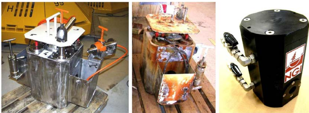
Figure 7-5 “Bright and shiny” instrument unit mainly in stainless steel prior to deployment (left) The same unit heavily corroded after 2 years deployment in seawater (middle). Corrosion “safe” instrument housing made of Delrin with outfitting in stainless (right)
