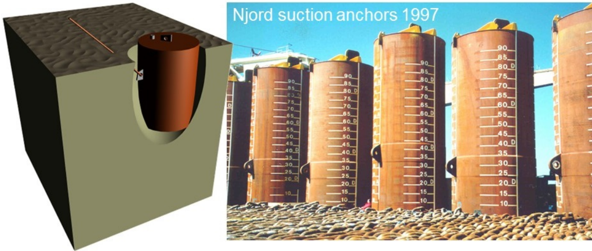
Figure 4-38 Suction anchors for catenary mooring to a large floater installed 1997 in the North Sea
