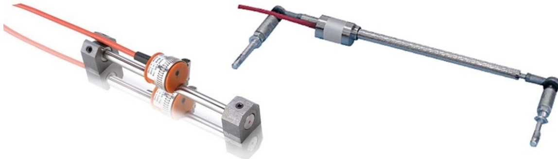
Figure 5-39 Vibrating wire strain gauge (left) and LVDT type of extensometer (right) often used as crack or joint meter (larger deformation range than a strain gauge)
