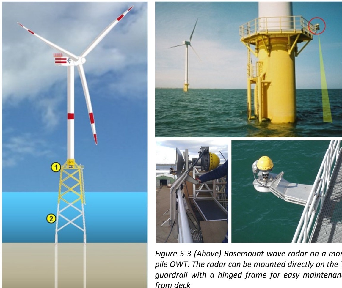
Figure 5-2 Left) Positions of Down looking microwave radar (1) or Up looking acoustic Doppler (2)
