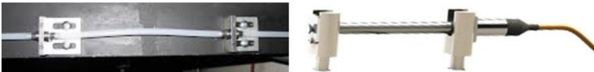
Figure 5-1 Example of long-gauge deformation sensors, fiber optic strain sensor by Smartech (left) and fiber optic extensometer by Opsens (right)
