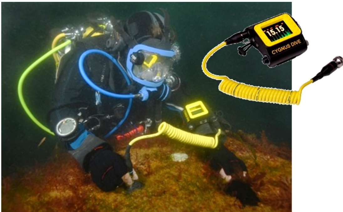
Figure 5-85 Diver operated ultrasonic Thickness Gauge from Cygnus instruments
