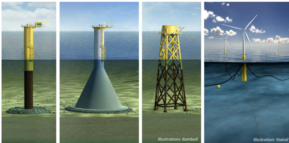
Figure 2-1 Main alternatives for Offshore Wind Turbine (OWT) foundations
