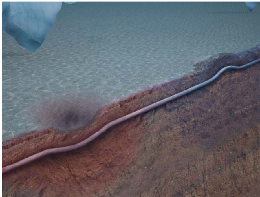
Figure 4-3: Thaw Settlement and Frost Heave
