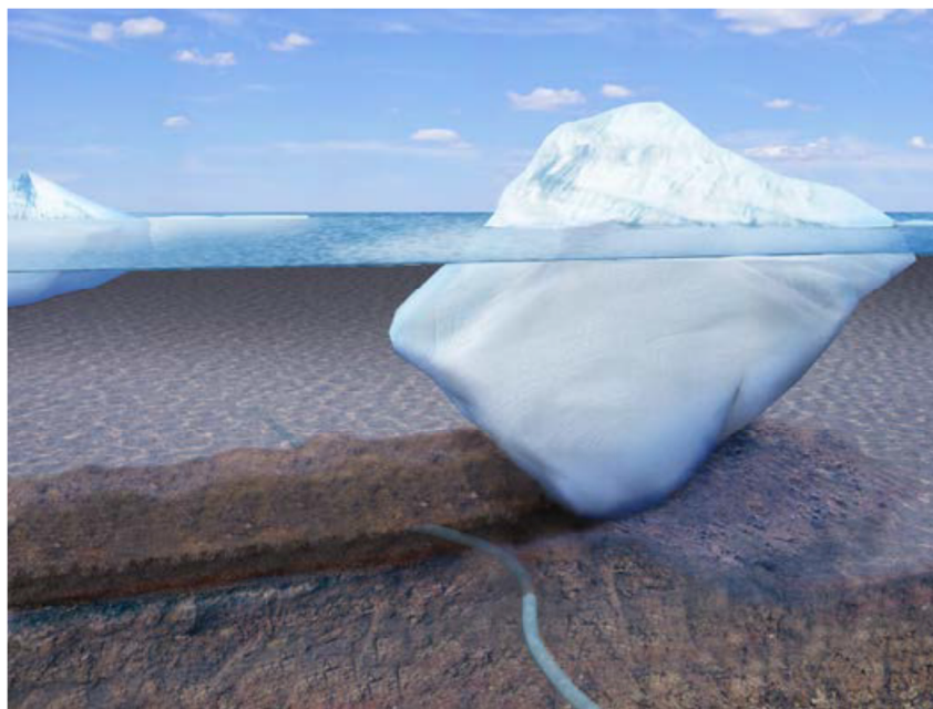
Figure 4-1: Ice Keel Scouring over a Pipeline
