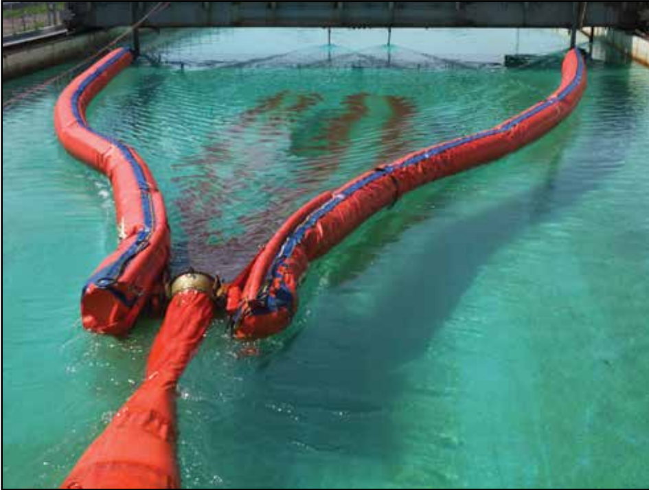
The improved Oiltrawl system encounters a slick of oil during performance testing at Ohmsett.
