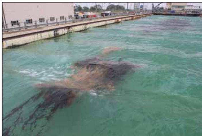
At left: Fresh crude oil was applied to the water surface in the Ohmsett test tank. To the right: A few minutes after dispersant was applied, the brown color is a visual indication of dispersed oil.
