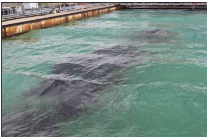
At left: Fresh crude oil was applied to the water surface in the Ohmsett test tank. To the right: A few minutes after dispersant was applied, the brown color is a visual indication of dispersed oil.
