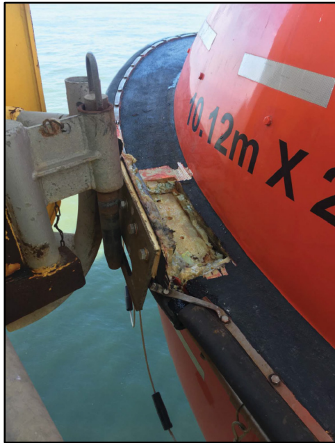
Lifeboat gripe plate after contacting a platform
