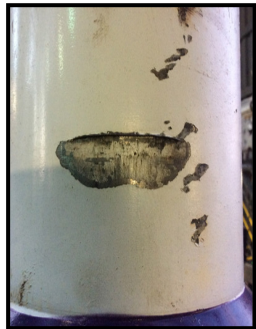
Figure 2. Damage to test tool assembly from BSR
