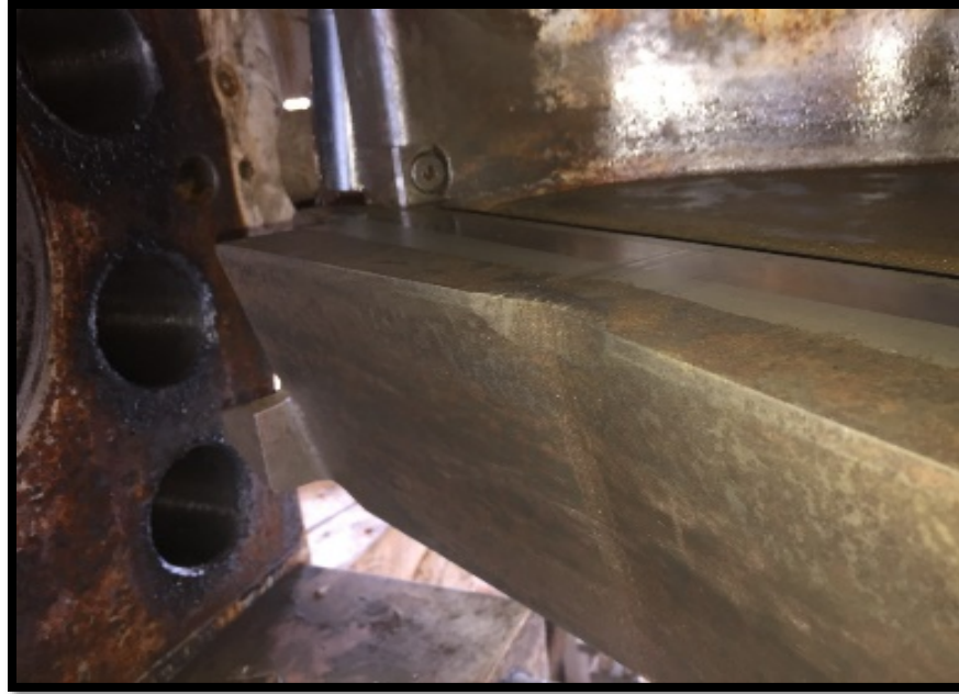
Figure 3. Damage to Blind Shear Ram after closing on the test tool
