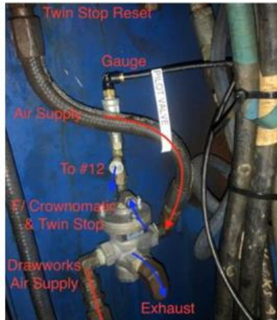
Emergency stop piloted valve
