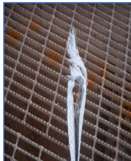
Figure 2. Broken FIBC Strap
