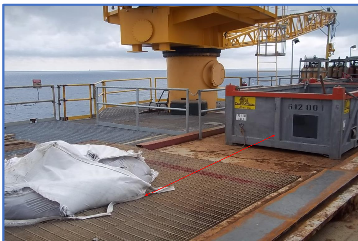
Figure 1. FIBC Load travel Path from the Cargo Basket to the Drop Zone 17 Feet Away
