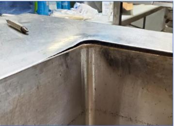
The crack on the surface of the steam table may have allowed steam to enter the enclosure and short out the electronics inside, causing a fire.
