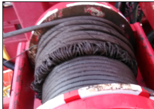
Damaged auxiliary line boom tip sheave
