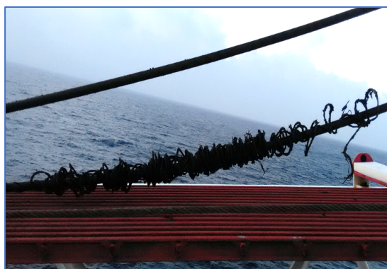
Damaged auxiliary line
