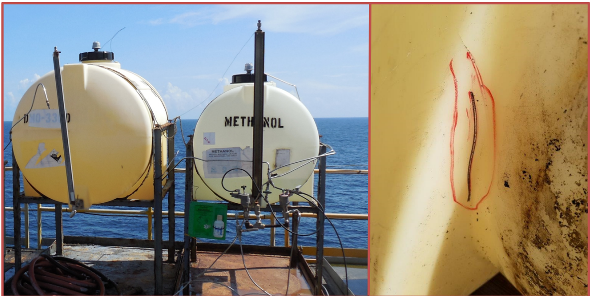
Location of storage tank (tank on left) at the time of the incident (left photo) and external view of the crack (right photo)
