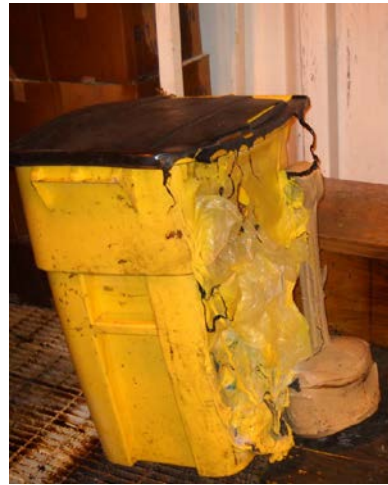
Damaged Trash Can and Cigarette Butt Container
