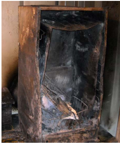
Damaged Freezer after fire.
