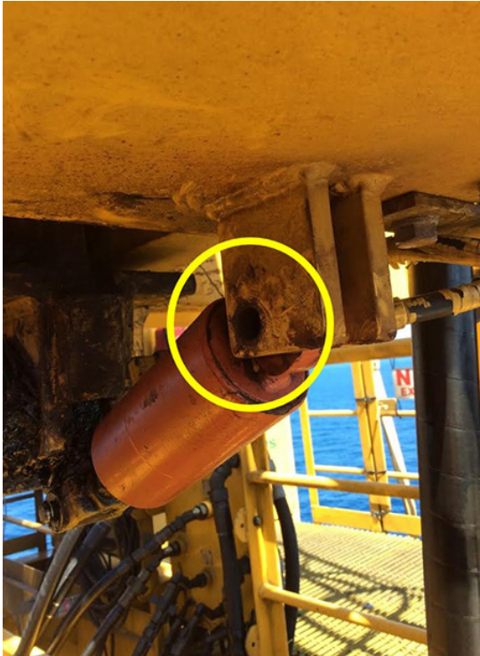
Location of the dislodged boom pawl pin is indicated by yellow circles.
