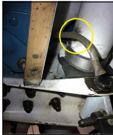
Figure 2. Lightning arcing on the aft strut
