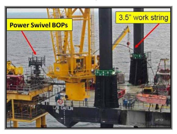
Recently, a loss of well control occurred as an OCS Operator was drilling out a combination surface cement/bridge plug during Plug and Abandonment (P&A) operations. The P&A operation was being conducted on the main deck of the platform, from a lift boat, using a power swivel, BOPs and crane.
