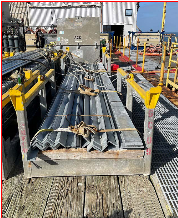
Load with incorrect weight recorded on manifest and wire rope with damage.
