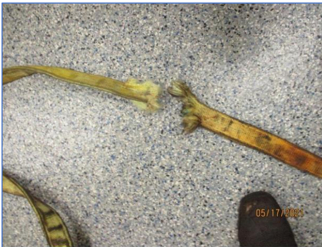
Figure 1. One of the Two Frayed / Parted Synthetic Slings from the Incident
