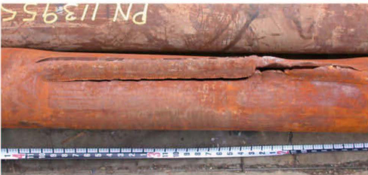
Damage in the drill pipe as received from the field.
