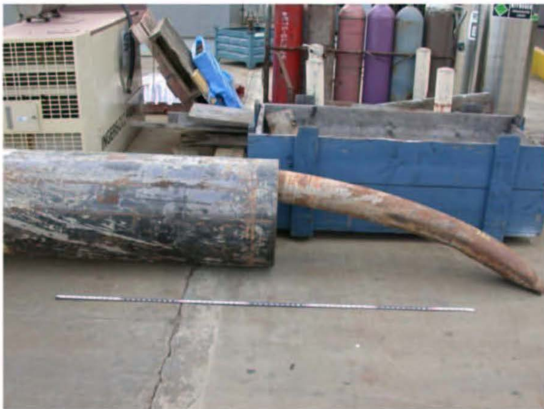
Upper damaged end of the 22-inch casing, showing the upper end of the drill pipe as delivered to lab.
