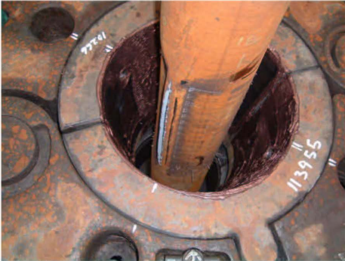
View of the crushed test pipe, following removal of the slips at lab.
