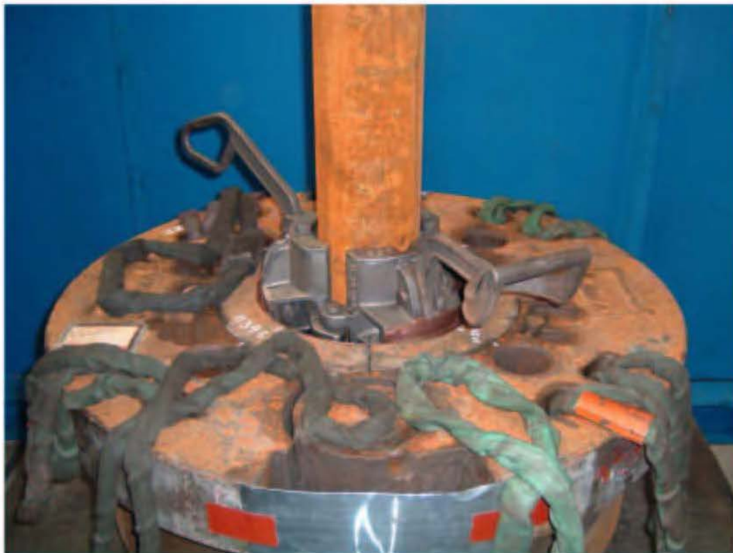
View of the slips and pipe before test at lab.
