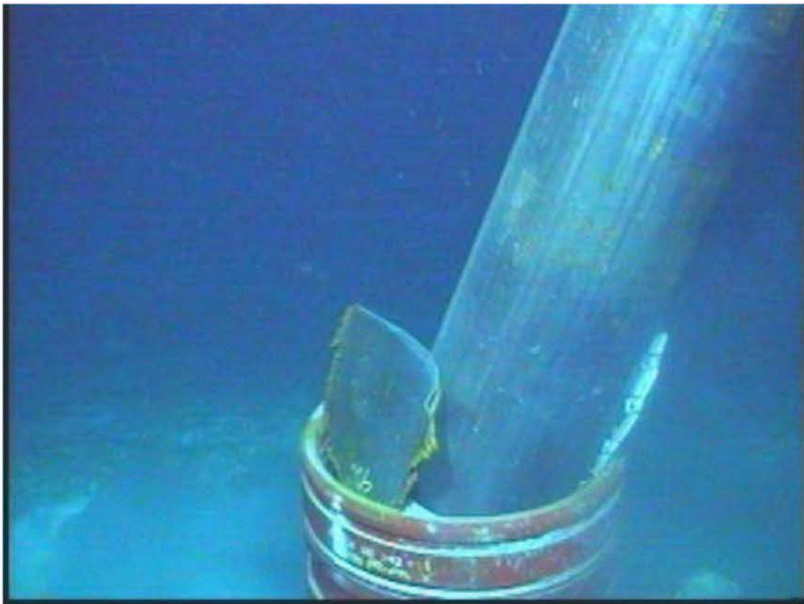
Parted and pinned casing on seafloor.
