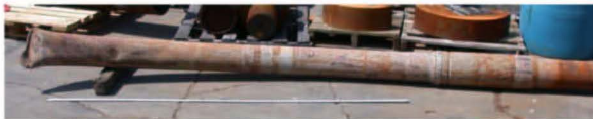
Upper end of the section of the drill pipe, after removal from the 22-inch casing.
