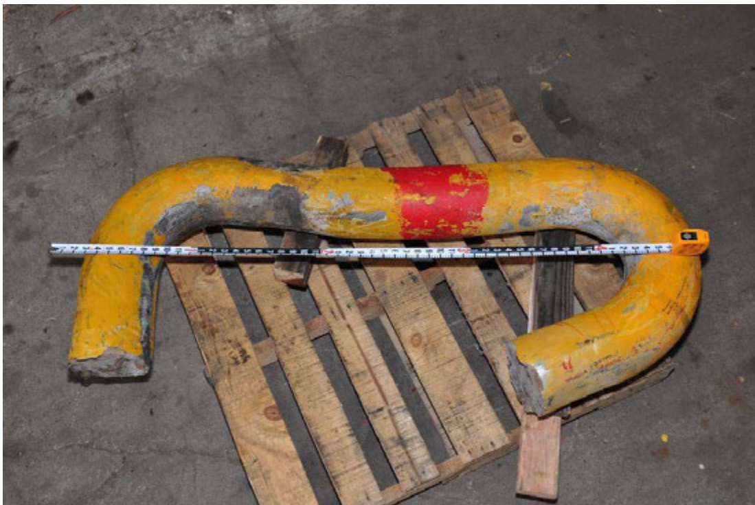
Failed Chain Link
