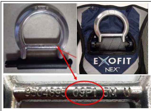
Defective DBI-SALA® ExoFit NEX™ Harness
