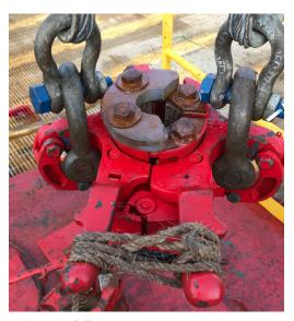
Tubular elevators installed with "C" plate upside down, which made the elevator dies size stamp hidden.
