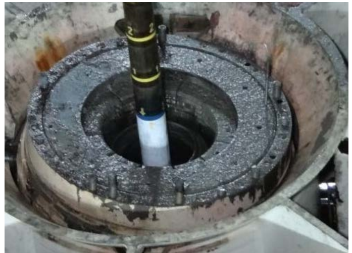
Lower half of failed LMRP Connector
