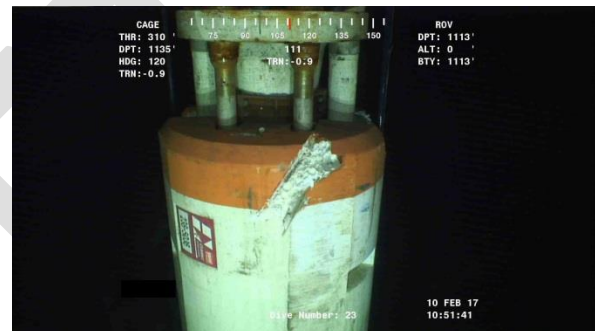
Left: moon pool flap on seafloor; Right: damage to riser buoyancy module
