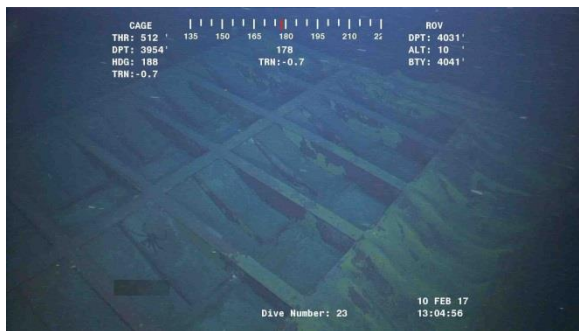
Left: moon pool flap on seafloor; Right: damage to riser buoyancy module
