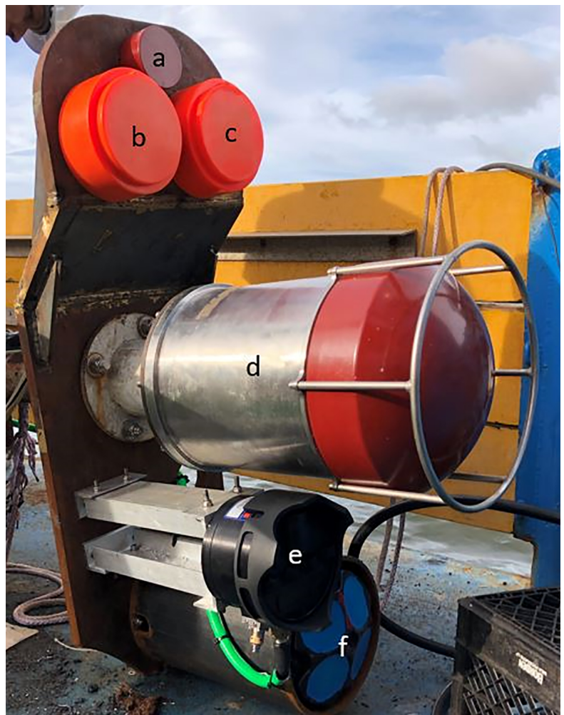
Figure 3.5. Acoustic sensors mounted on overboard pole of R/V Brooks McCall . Sensors are labeled as Simrad EK80 splitbeam transducers operated at 70 kHz (a), 120 kHz (b), 200 kHz (c), the HiPAP USBL (d), Kongsberg M3 multibeam echosounder (e) and RDI ADCP (f).
