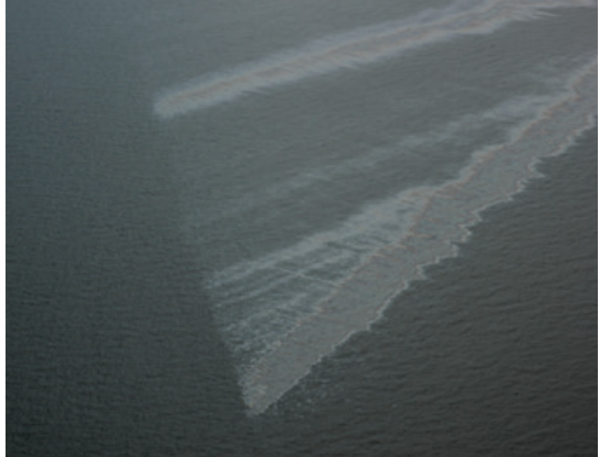
Figure 1.3. Persistent oil slicks originating from the erosion pits under the platform jacket.
