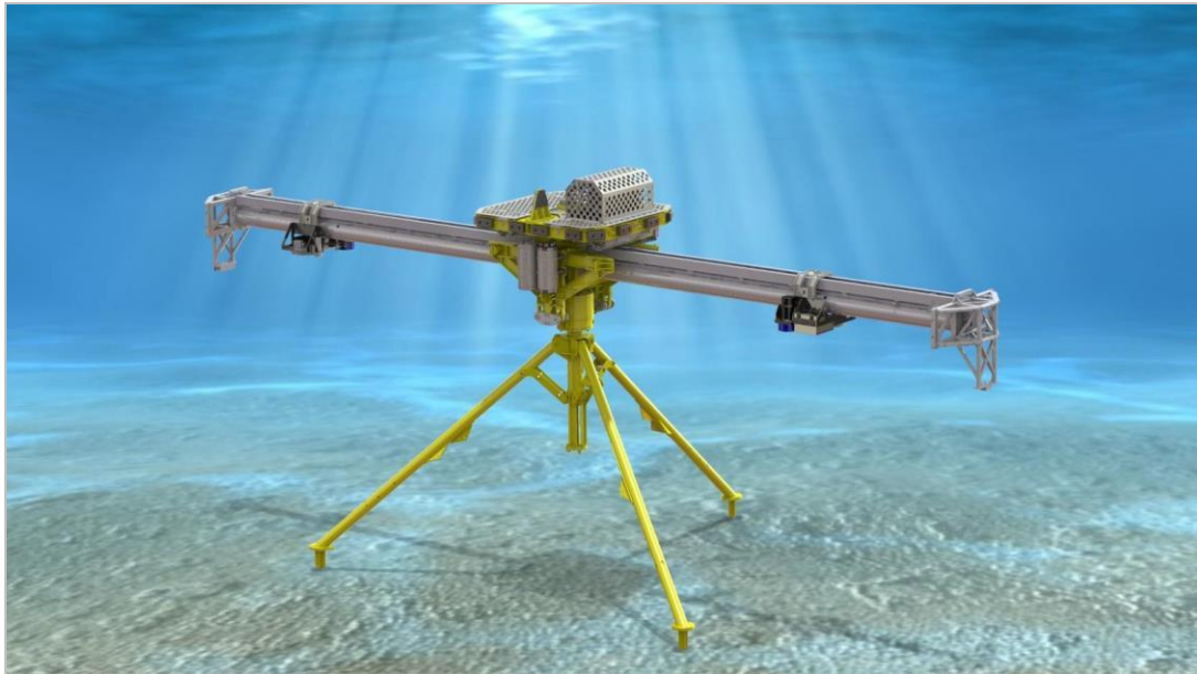
Figure 7 - Acoustic Corer – normal operation on tripod legs
