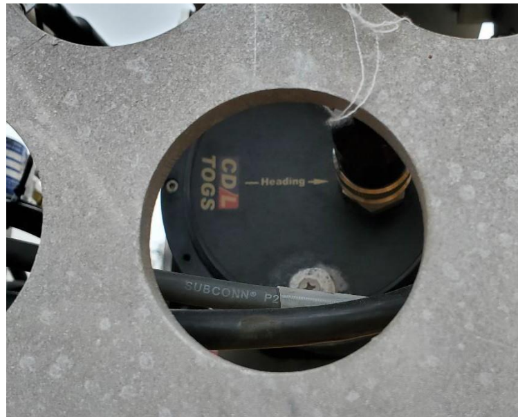
Figure: Image showing incorrect orientation of TOGS, Mississippi Canyon Campaign 2019
