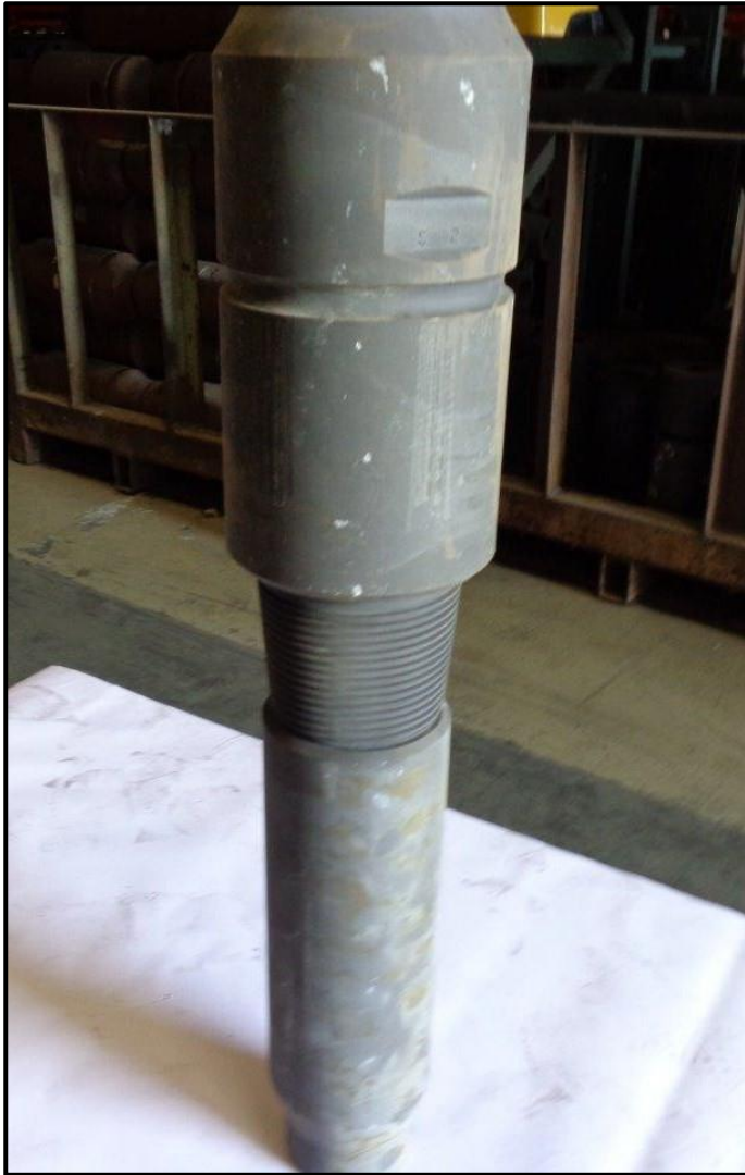
Figure 22: Top drive 5-in pin above 3 ½-in box
