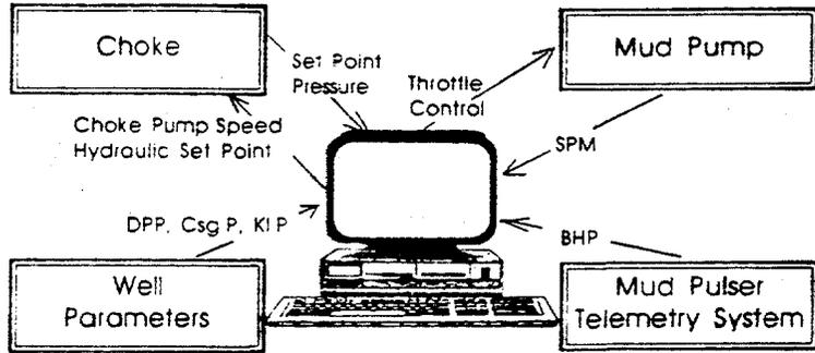
Figure 11 - Computer Control for Automated Well Control Safety System
