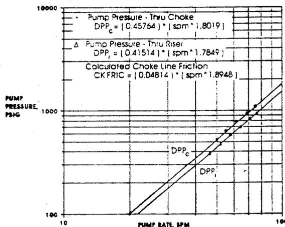
Figure 9 - Typical Subsea Pump Flow Rate vs. Pump Pressure Curve Fit
