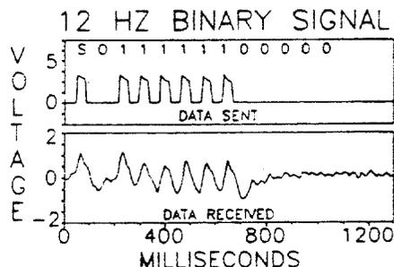
Figure 10 - Typical Fluidics Mud Pulser Encoded Data
