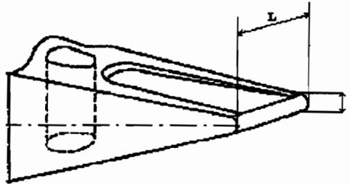
**Figure 1. Wedge type new excavator tooth geometry.**
