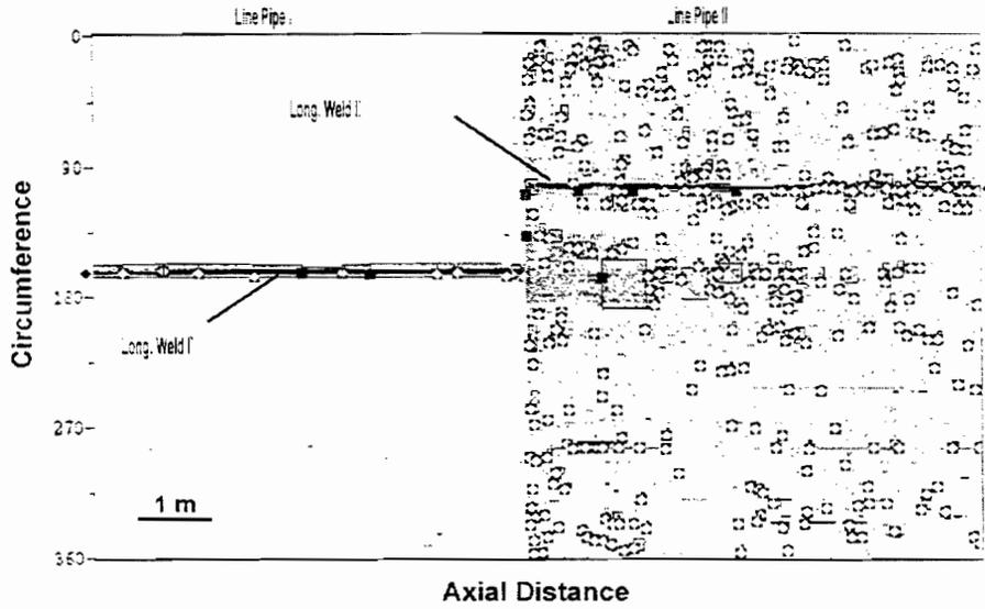
Figure 10 C-scan from UltraScan CD data showing part of clean line pipe (left) and part of line pipe containing numerous inclusions & laminations (right).
