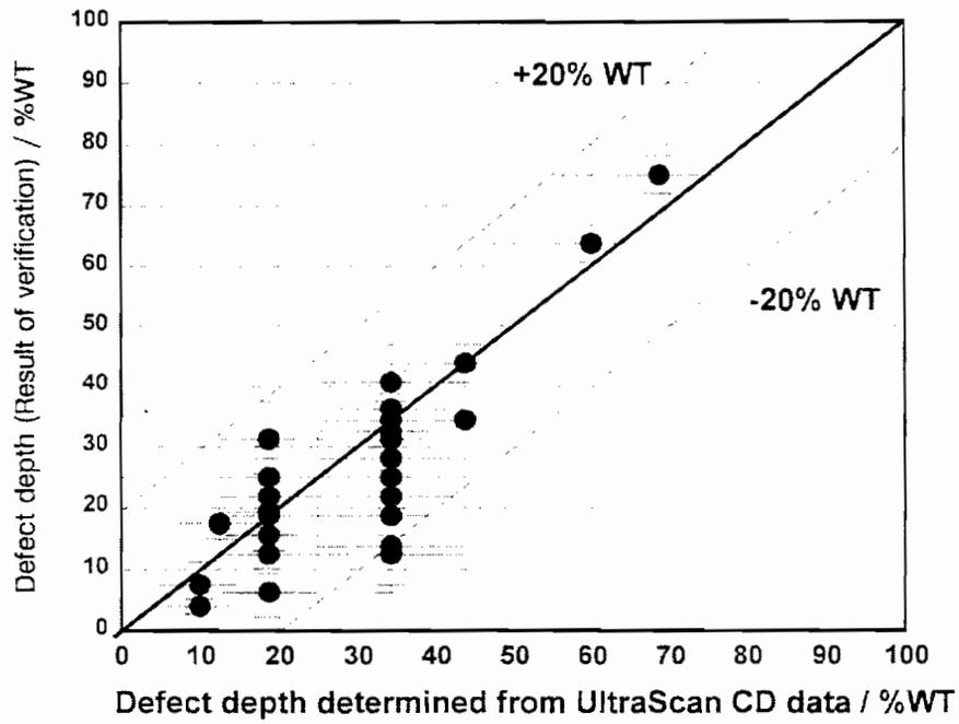
Fig. 8: Comparison between crack depth as determined from UltraScan CD data and the results obtained by manual inspection
