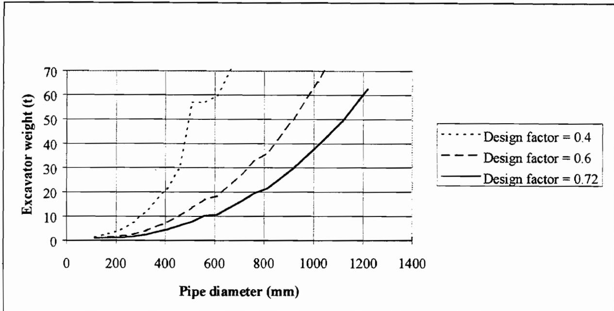
**Figure 2 : Puncture proof excavators in the vicinity of gas transmission pipes as a function of diameter.**
