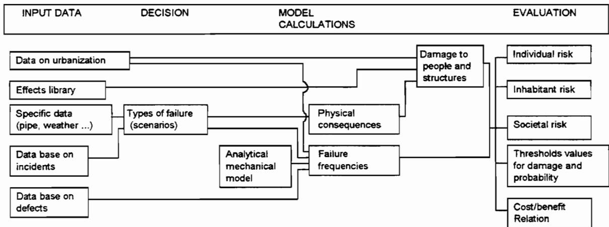
Figure 6. Logic chart for the safety assessment methodology
