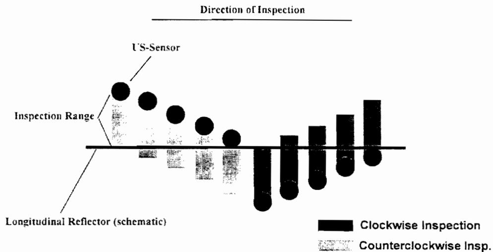
Fig. 3: View of sensor arrangement illustrating the multiple wall coverage
