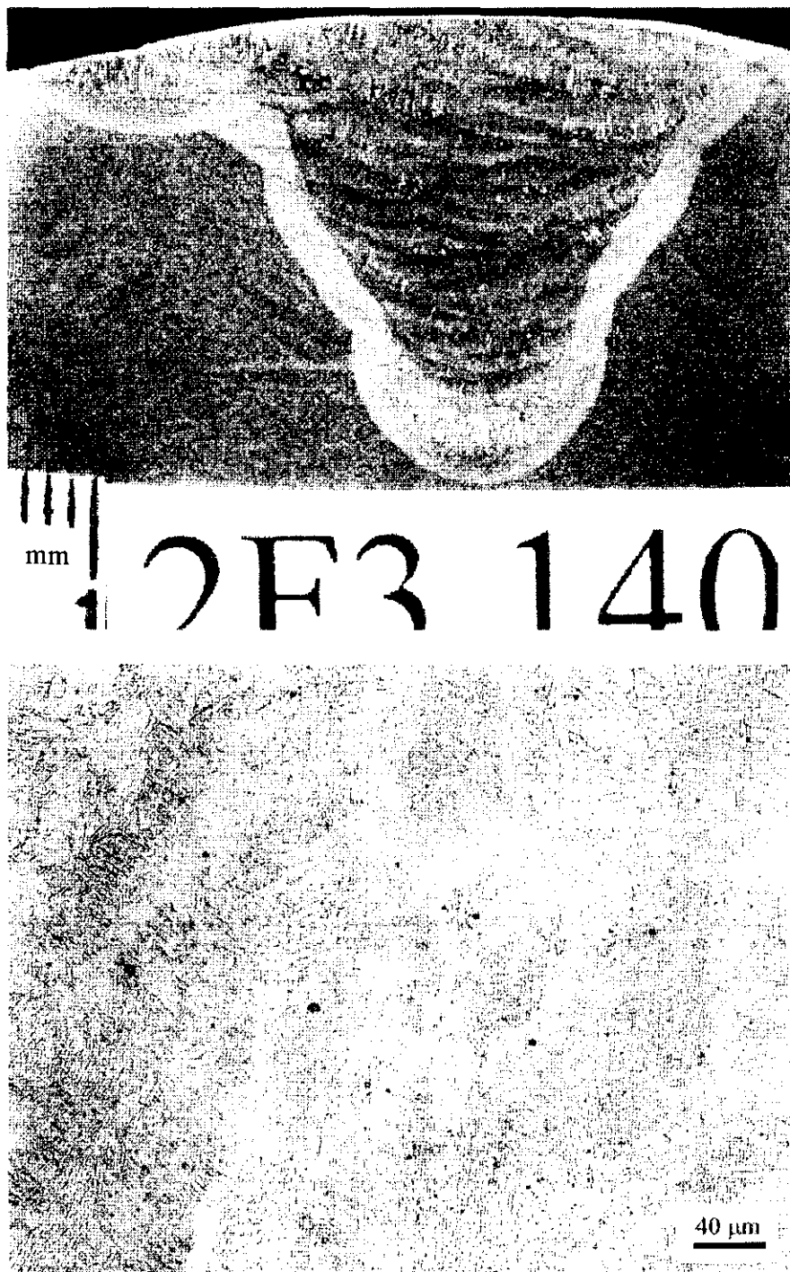
Figure 37: Macro-section and top bead microstructure of the 2F3 140 ft (43 m) V-groove weld.
