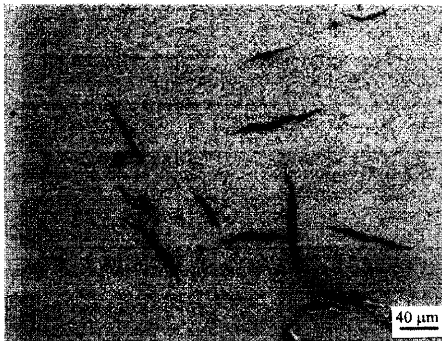
Figure 58: Micro-cracking in 1F3 as-deposited weld metal (top) and 2F3 reheated weld metal (bottom).
