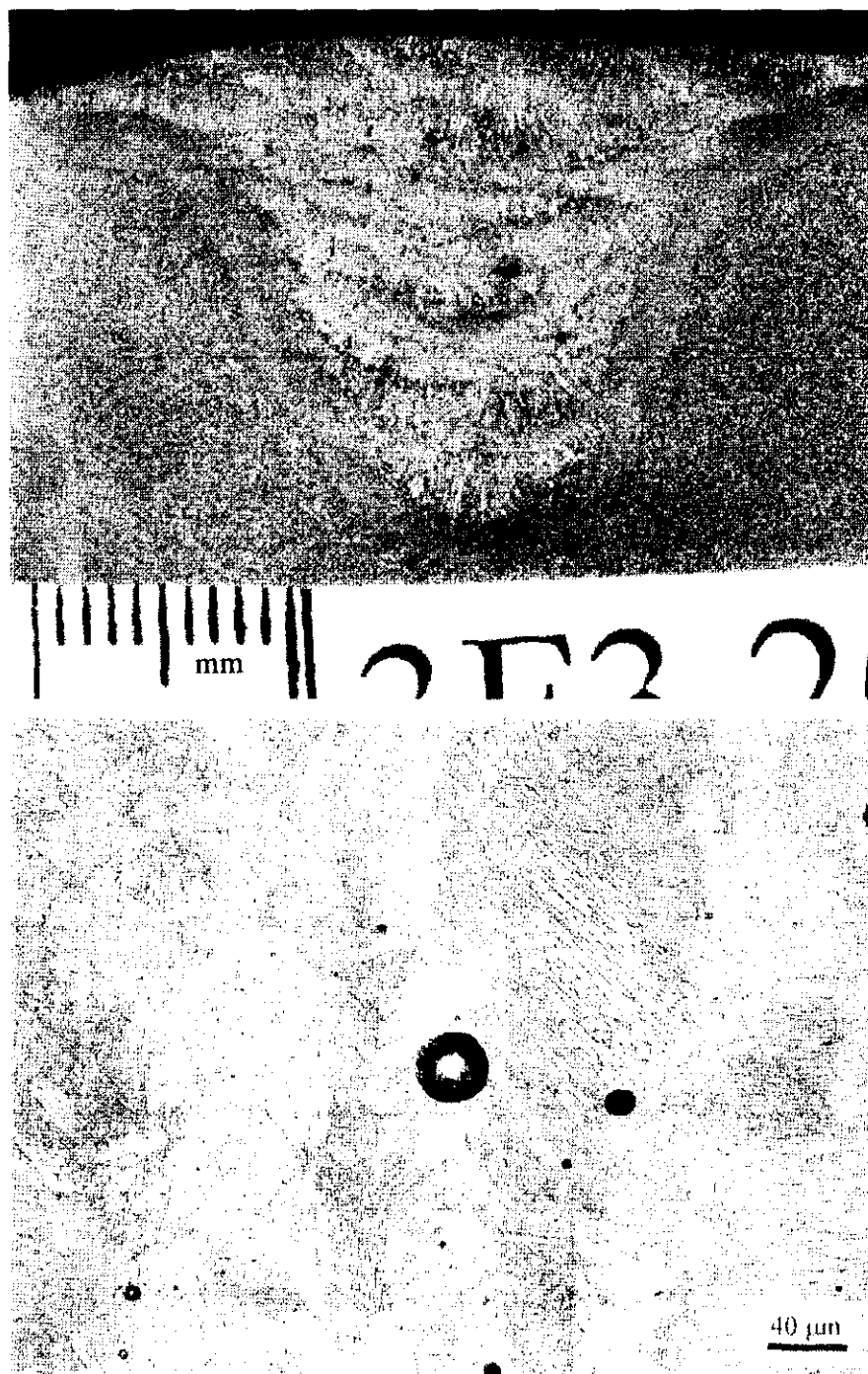
Figure 38: Macro-section and top bead microstructure of the 3F3 200 ft (61 m) V-groove weld.
