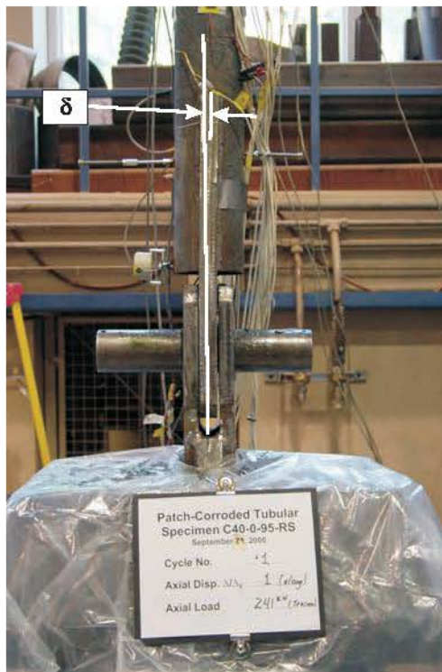
Figure 5.102 View of End Plate Bending (Load Step -2), Specimen C40-00-95-RS
