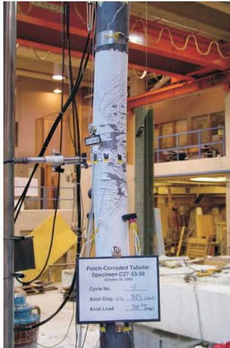
Figure 5.71 Yielding at Mid-height (Load Step -1), Specimen C27-33-58
