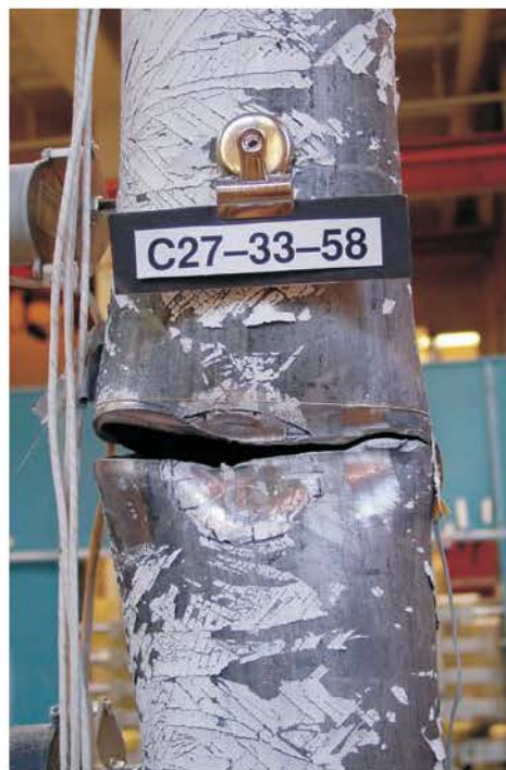
Figure 5.76 Through Thickness Cracking Across Local Buckle (Load Step +7), Specimen C27-33-58
