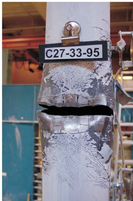
Figure 5.86 Side View of Through-Thickness Cracking at Edges of Local Buckle (Load Step +3), Specimen C27-33-95
