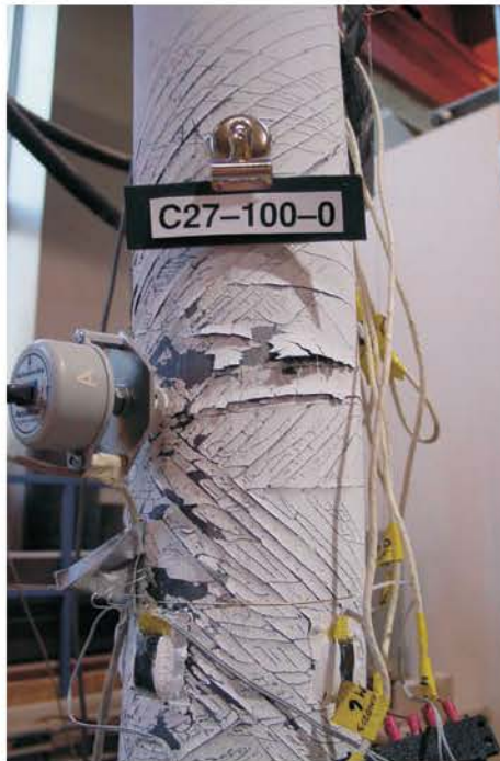
Figure 5.17 Side View of Yielding at Mid-height (Load Step -1), Specimen C27-100-0
