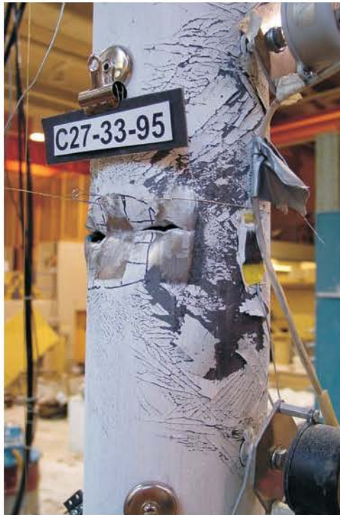
Figure 5.86 Side View of Through-Thickness Cracking at Edges of Local Buckle (Load Step +3), Specimen C27-33-95
