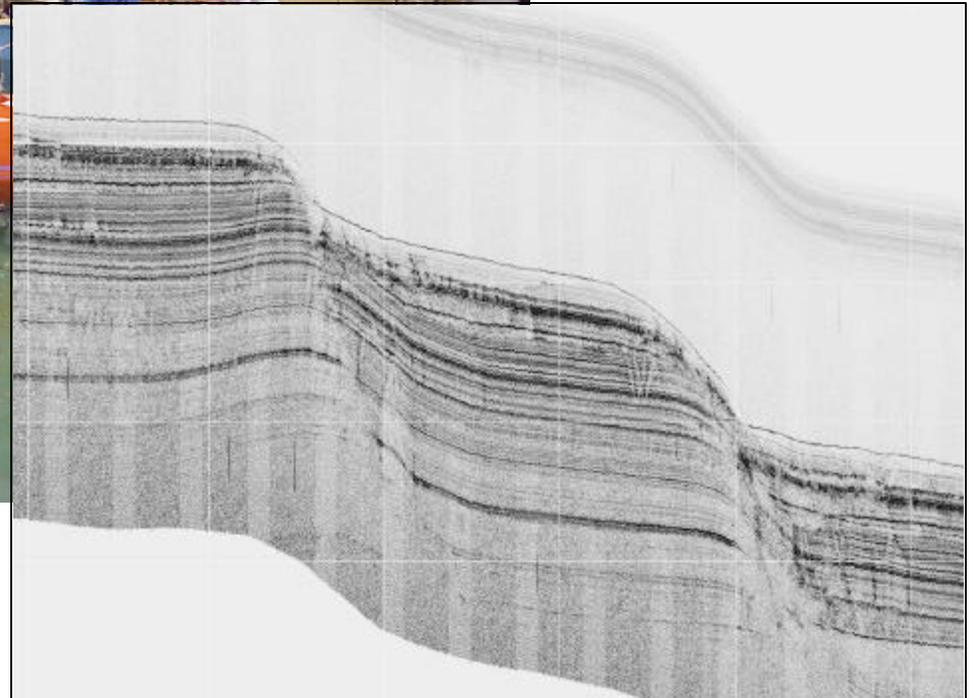
AUV Chirp Profiler
