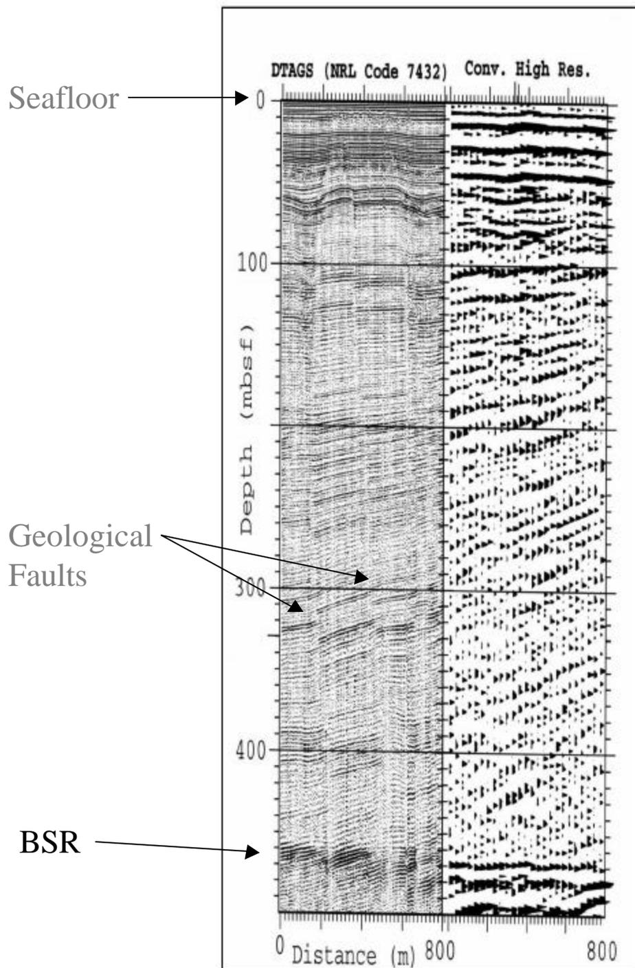
The order of magnitude improvement in both vertical and lateral resolution of DTAGS data (250-650 Hz) over conventional high-resolution single-channel air gun data (10-220 Hz), Line 31 from Katzman et al., 1994 is clearly shown in this figure.
