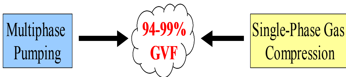
Figure 3.23: Approaches to Wet-Gas Compressor Development
