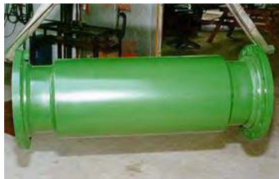
Figure 5.10: North Sea MFC designed for 10000 BOPD 56 .
