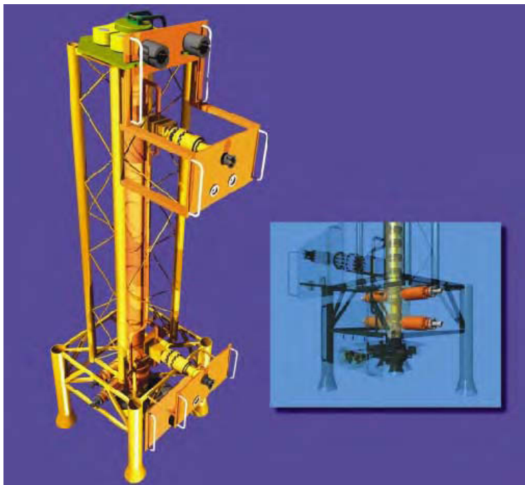
Figure 5.6: Equipment for single trip pigging 56 .
