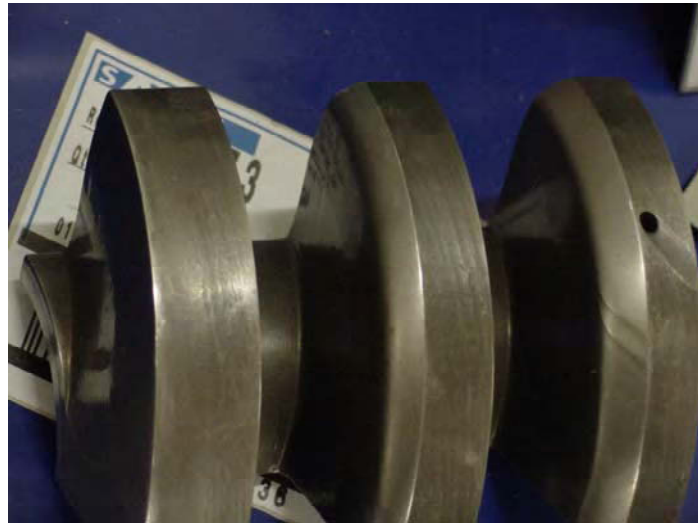
Figure 3.31 – Wear Caused by Sand Production
