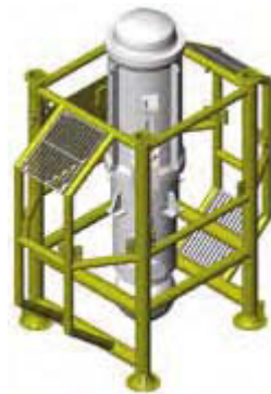
Figure 2.11: Schematic of a subsea gas compressor 5 .
