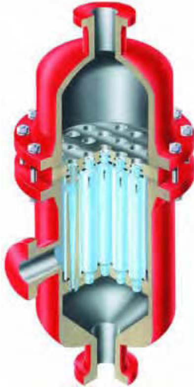
Figure 4.6: Cutout of a desanding multi-cyclone 49 .
