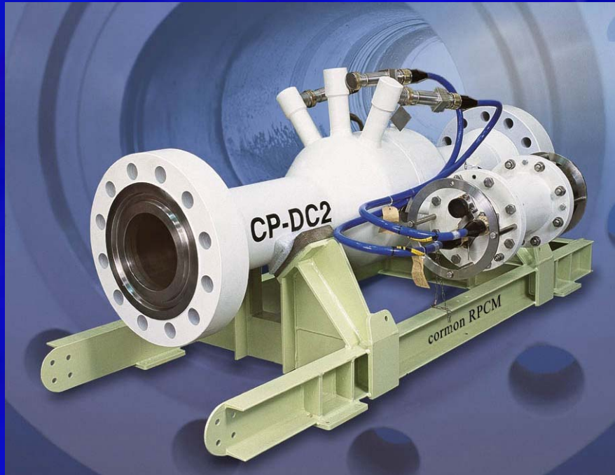
1 Cormon Limited, RPCM (Ring Pair Corrosion Monitor) - sensors exposed to flow measure internal wall loss
