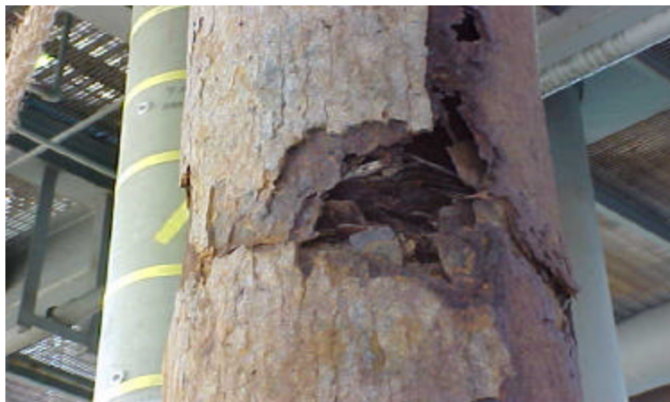
Figure 15.2: Photo of heavily corroded conductor
