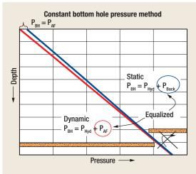
Fig. 4. The constant bottomhole-pressure variation of MPD uses lower-density drilling fluid and imposes backpressure when static to equalize annular friction pressure.
