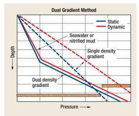
Fig. 7. The dual-gradient variation uses two density gradients, a lower density on top and higher density on the bottom.
