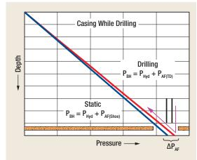
**Fig. 6.** In casing while drilling, pumping manages friction pressure through the casing drillstring.
