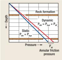
Fig. 1. Ideally, static and dynamic pressures are within formation-pressure and fracture-pressure windows.
