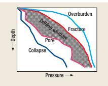
Fig. 2. Land-based and shallow-water drilling using single-density drilling fluid have a wide drilling window.
