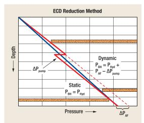
Fig. 8. To create a reduction in ECD, a downhole pump produces a pressure differential that modifies the annular pressure profile.
