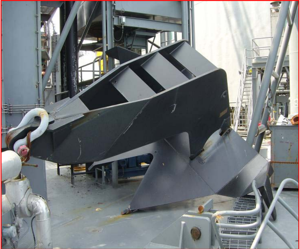
Figure 8.13.1: 5-ton anchor was racked on the exterior of the hull 50 feet above the sea before the storm
