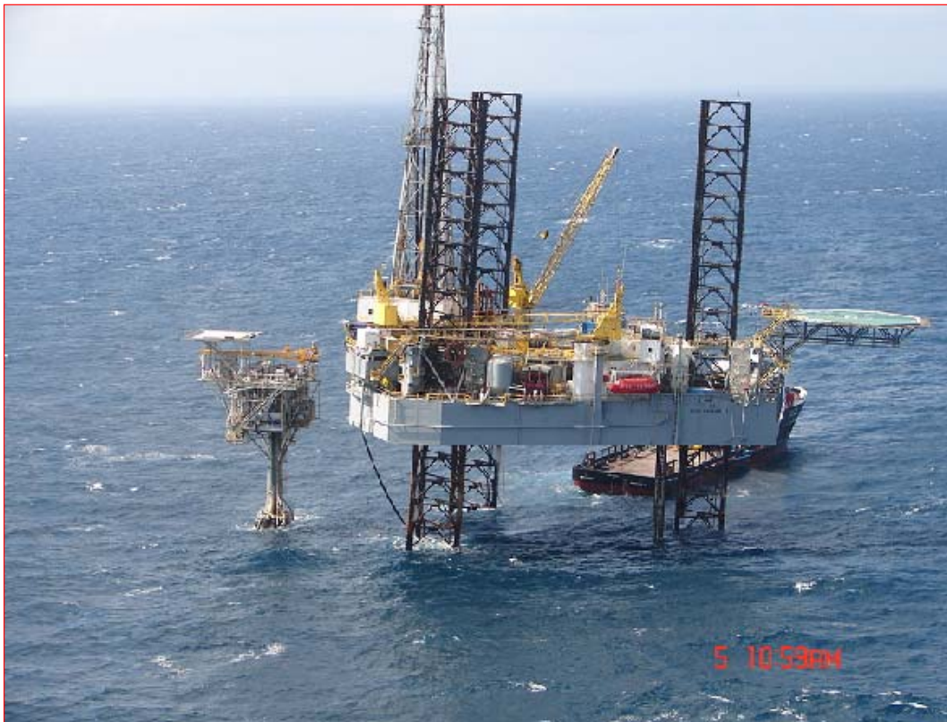
Photo: 9.17.2 When attempts were made to jack the rig down, extreme loads were imparted to the legs at the transition to the hull/leg guides using further leg cracks.
