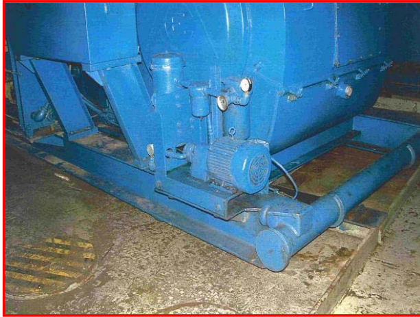
Photos 9.15.8: Mud Pump moved off foundation due to rig movement;
